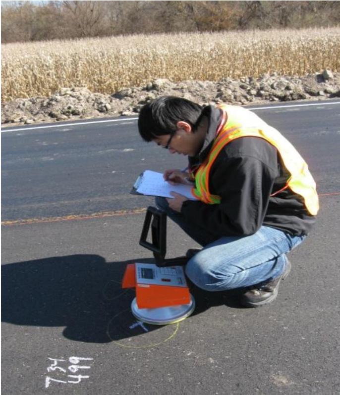
Figure 3.5: PQI model 301 taking measurements
