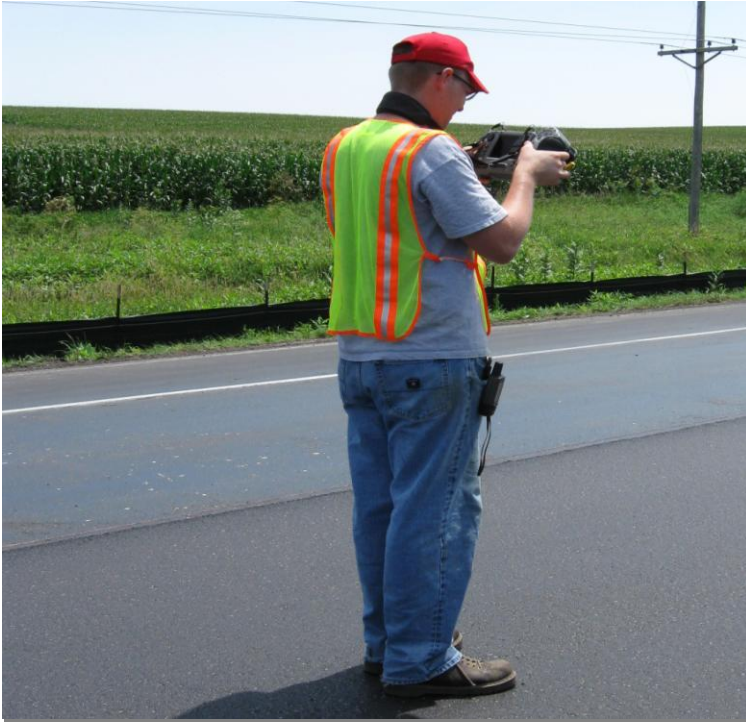
Figure 3.1: Use infrared camera to choose density testing location
