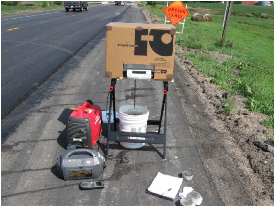
Figure 3.6: On-site set up for core measurements
