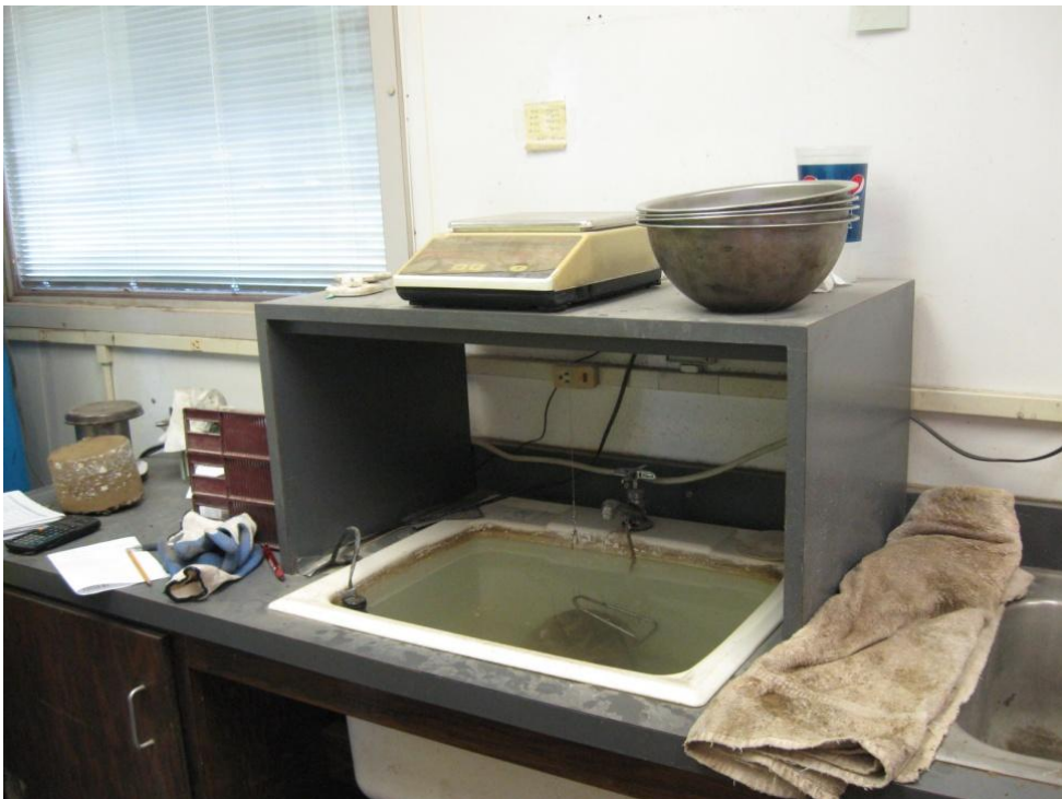
Figure 3.6: On-site set up for core measurements
