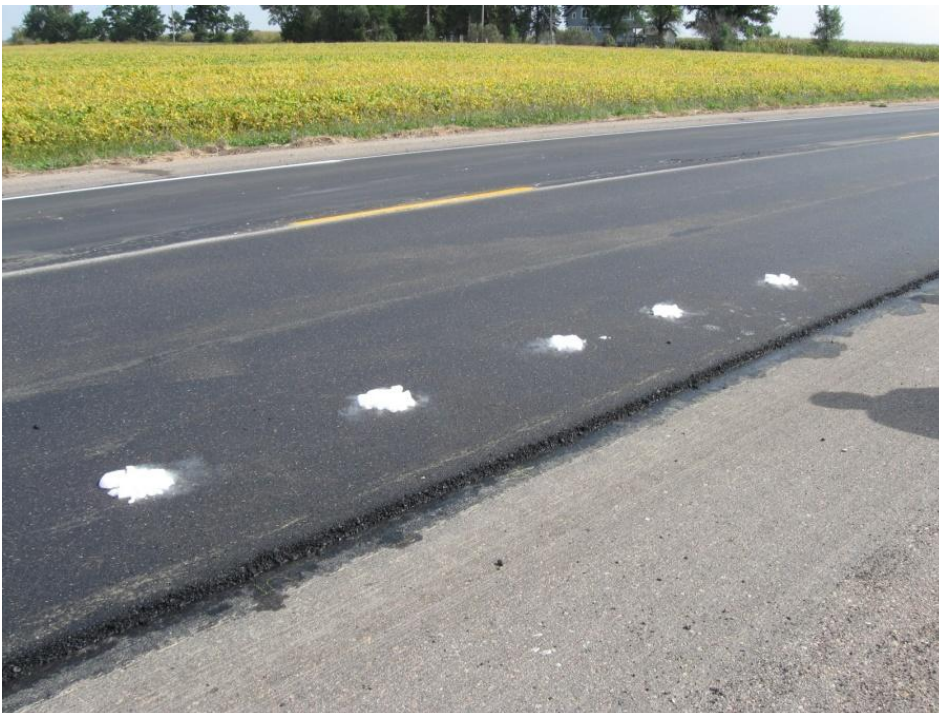
Figure 3.1: Use infrared camera to choose density testing location
