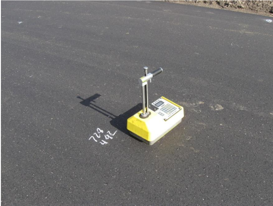
Figure 3.4: Nuclear Gauge is shown measuring density
