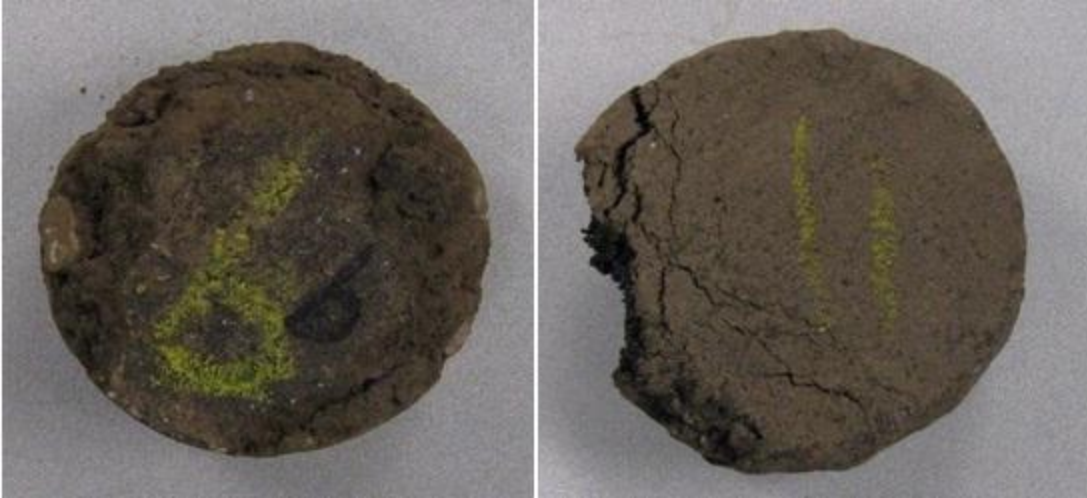
Figure 4.1: Example of a rejected core
