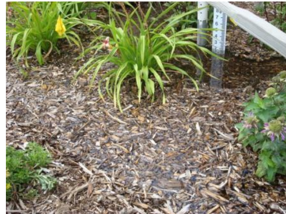
Figure 48. Floating mulch (characteristic of almost every garden) and water lapping against berm face. Transducer and staff gage in background.
