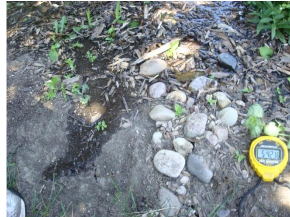
Figure 44. "Full" garden showing overflow across the berm near the designed outlet. Note: overflow had occurred in numerous other spots before this, indicating inappropriate
