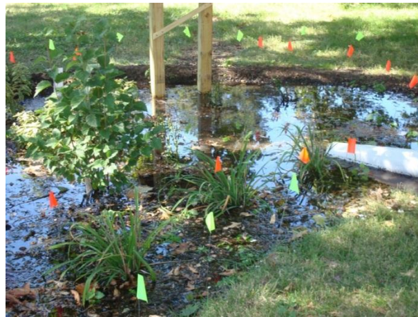
Figure 11. Garden after second simulated storm showing perimeter flags for each event (differentiated by color).
