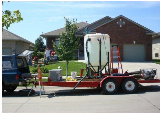
Figure 8. (a) Storm water runoff system schematic. (b) Image of simulator at study site.
