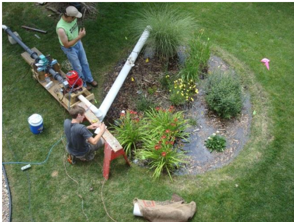
Figure 39. Bird's-eye-view photograph of full rain garden just after simulation was stopped pending overflow.
