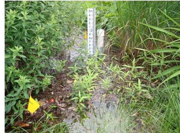
Figure 32. Full rain garden with outflow escaping over grass berm. Stilling well and staff gage also shown.
