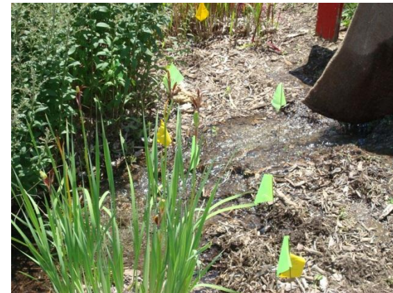
Figure 36. Influent from the simulator system is shown entering through the burlap sack (used for erosion control). Note the hydraulic flow path to outlet indicates poor retention.
