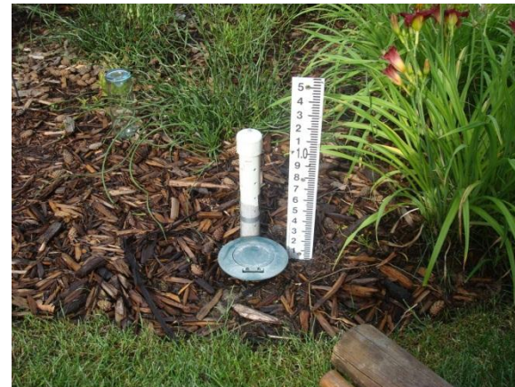
Figure 40. Data collection devices at the inlet of the rain garden. The inlet is a pop-up riser inlet conveying roof runoff.
