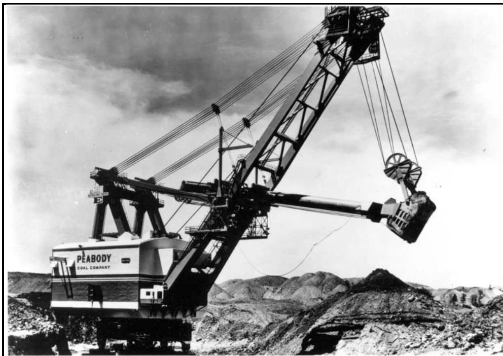
Figure 4-26. "The world's largest mobile land machine." The stripping shovel built by Bucyrus-Erie for Peabody's Tebo Mine. See Figure 4-4 for size comparison of the bucket. Photo courtesy of the Henry County Historical Society.
