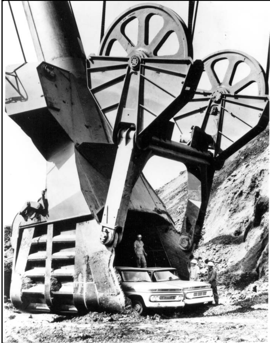
Figure 4-5. Tebo Mine—Bucket from shovel—in northeastern Henry County, circa 1960. The giant dipper on the Bucyrus-Eric stripping shovel picked up almost 200 tons of rock and dirt with every shovelful. Photo courtesy of the Henry County Historical Society.
