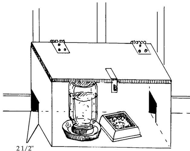
Fig. 16. A homemade rodent bait station can contain liquid as well as solid baits.
