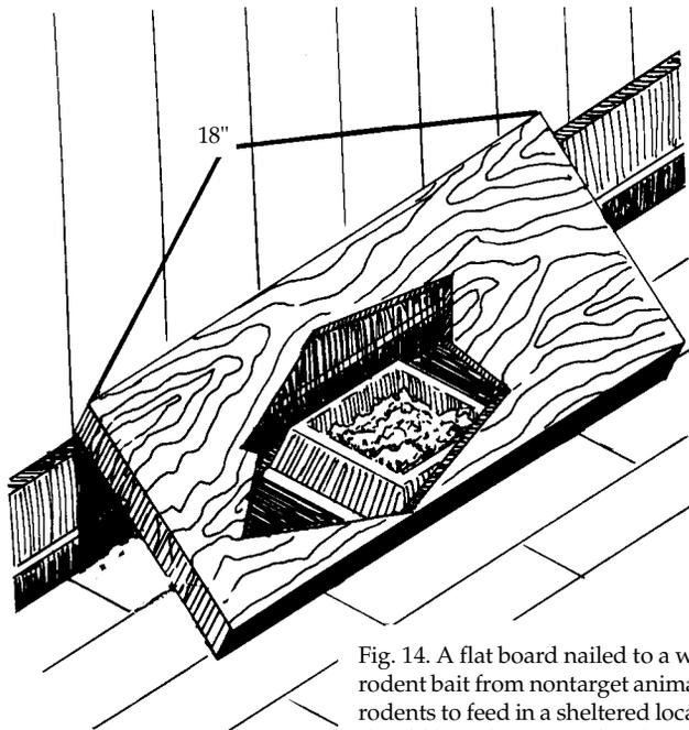
Fig. 14. A flat board nailed to a wall protects rodent bait from nontarget animals and allows rodents to feed in a sheltered location. The board should be at least 18 inches (46 cm) long to keep pets and children from reaching the bait.
