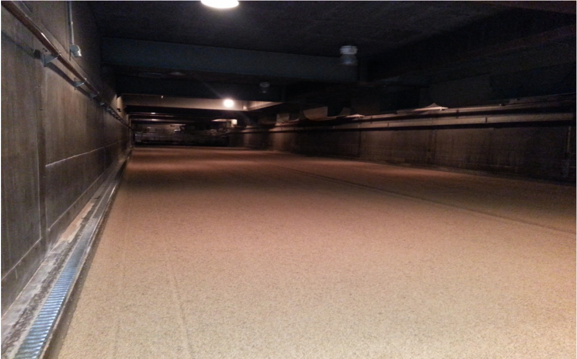
Figure 2.6 – Kiln drying down green malt. Green malt is evenly spread across the floor, and hot air is blown up through the grain bed. Photograph taken by Haley Oser at Golden Malting in Golden, CO.
