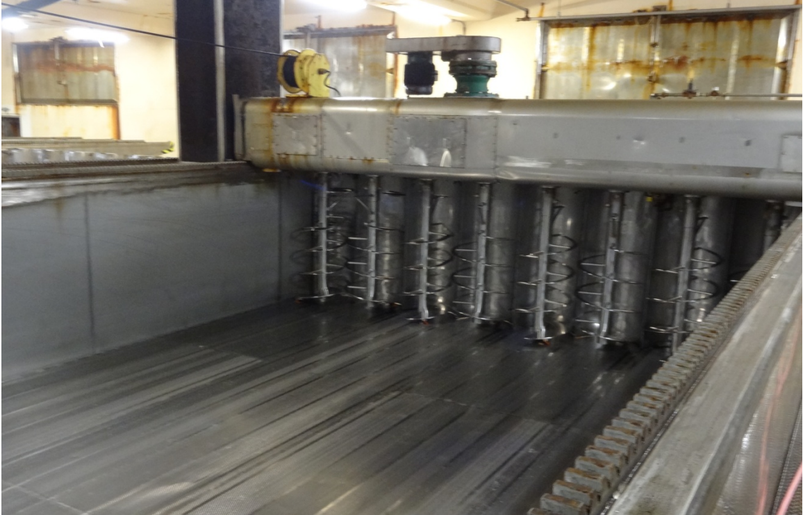
Figure 2.5 – Saladin box demonstrating large vertical open augers. Carriage moves across the top of the grain bed turning the grain. Photograph taken by Haley Oser at Golden Malting in Golden, CO.
