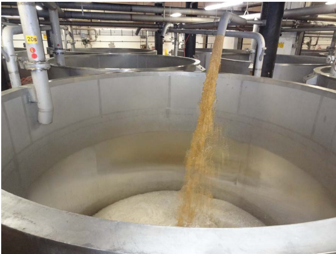
Figure 2.1 – Filling Steep Tank with slurry (water and barley). Photograph taken by Haley Oser at Golden Malting in Golden, CO.
