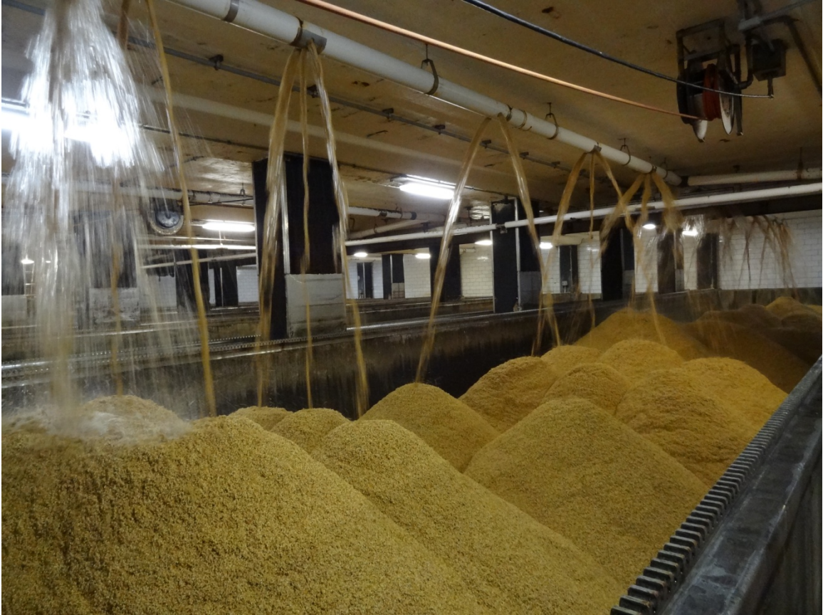
Figure 2.2 – Steeped grain being transferred to the germination bed. Photograph taken by Haley Oser at Golden Malting in Golden, CO.
