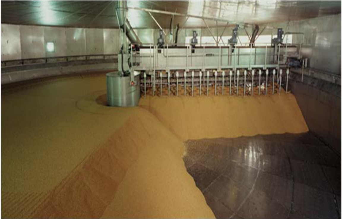
Figure 2.4 – Circular construction germination bed. Photograph courtesy of Mont Stuart.
