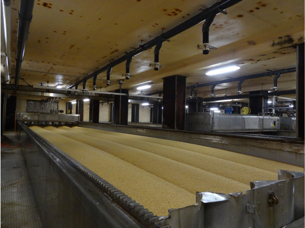
Figure 2.3 – Saladin Box (germination bed). Photograph taken by Haley Oser at Golden Malting in Golden, CO.
