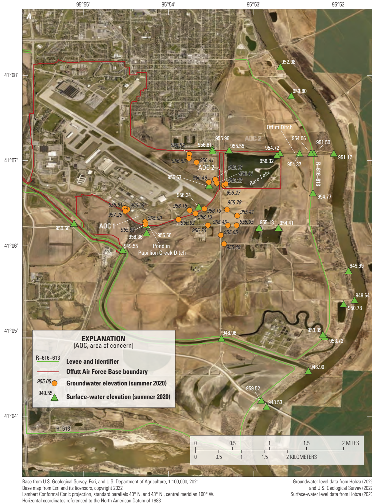
Figure 6. (A) Measured groundwater- and surface-water elevations and (B) locations of measured water levels and estimated groundwater flow direction from the late summer synoptic water-level survey data on and near Offutt Air Force Base, Nebraska, August 31–September 3, 2020. Groundwater-level elevations are shown in black labels and surface-water elevations are shown in white labels in figure 6A.
