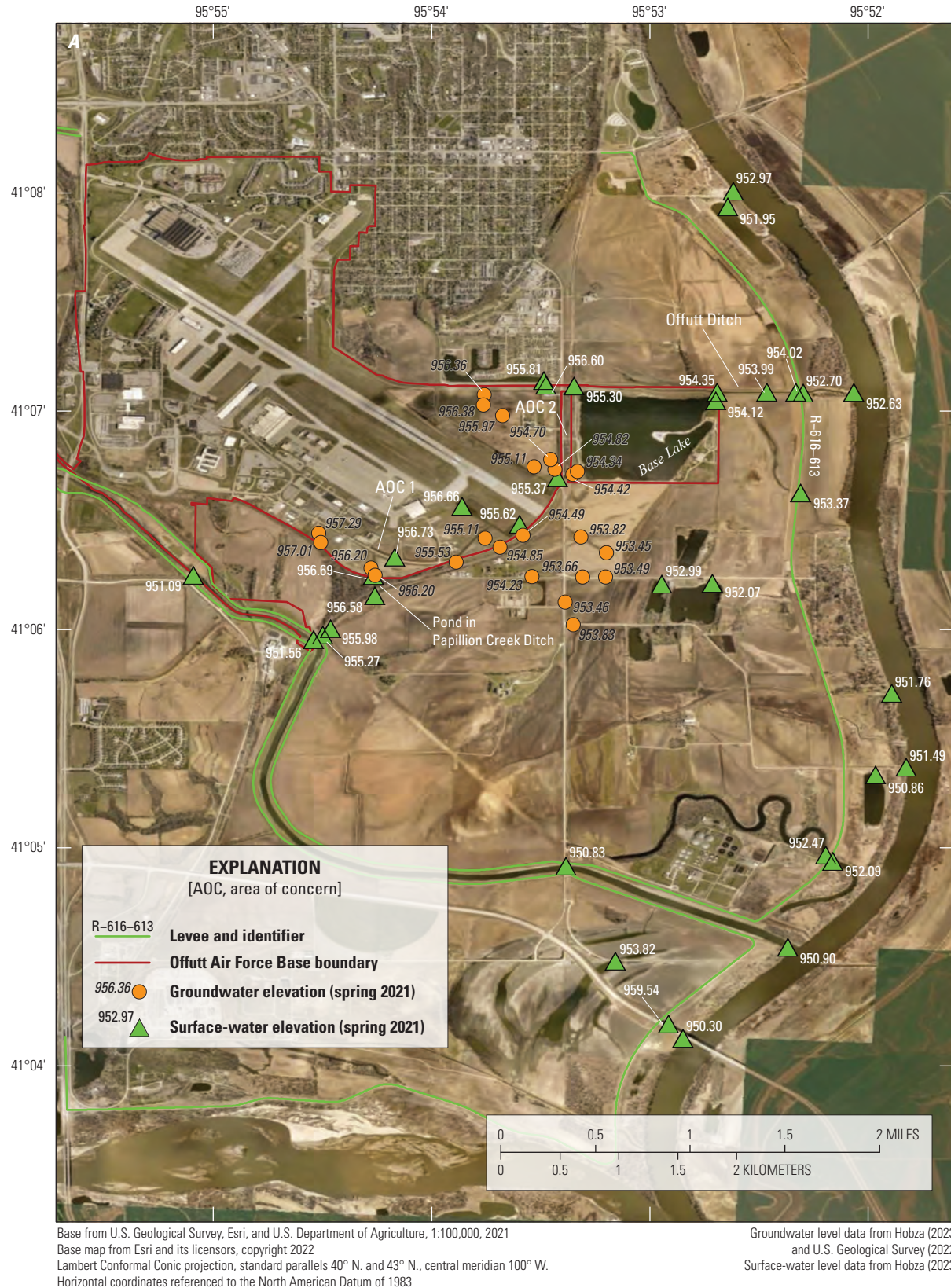
Figure 7. (A) Measured groundwater- and surface-water elevations and (B) locations of measured water levels and estimated groundwater flow direction from the late spring synoptic water-level survey on and near Offutt Air Force Base, Nebraska, May 3–5, 2021. Groundwater-level elevations are shown in black labels and surface-water elevations are shown in white labels in figure 7A.
