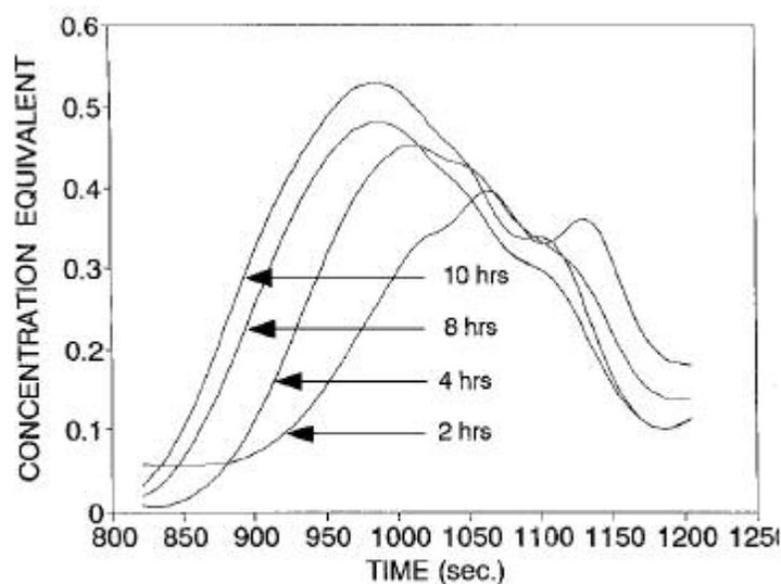
**Fig 7 ZGlu OH/DGEBA/PTS polymerization dynamics prior to gelation 110°**
