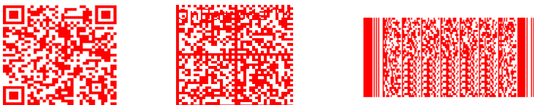
FIG. 2: Samples of eCodes (QR, Datamatrix, and PDF417)
