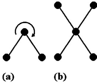
FIG. 1. Simple real-space illustration of Dzyaloshinskii-Moriya (DM) interactions: (a) nonzero interaction in magnets with low symmetry and (b) absence of DM interactions for crystals with inversion symmetry.
