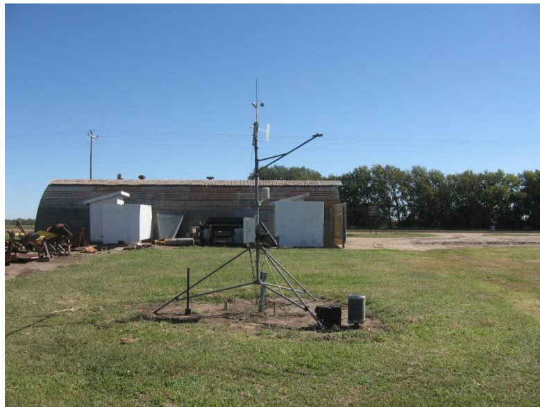
Figure 2.3. Weather station located at Scandia, KS. The weather station is located in direct proximity to a building. ( http://wdl.agron.ksu.edu/metadata.php )
