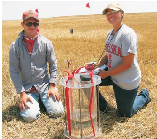
Brian Twombly (undergraduate BSEN) and Shannon Rose Bates (undergraduate AGEN) assisted Dr. Eisenhauer with research in the Republican River Basin in Kansas. They used this Cornell infiltrometer to simulate rainfall and measure water infiltration.
