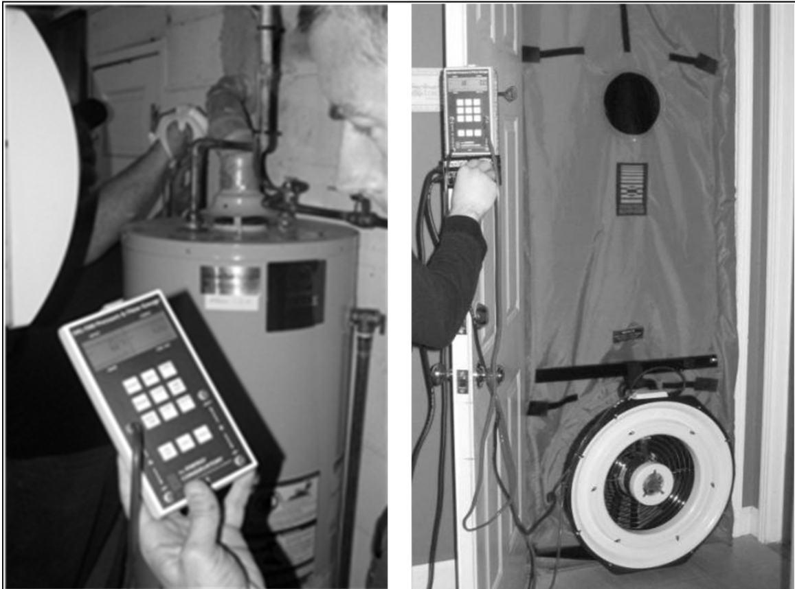
Figure 15 – CAZ and blower door testing
