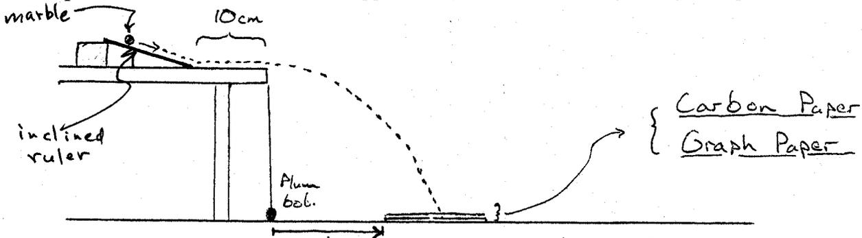
2. Roll the marble down the ruler (starting from rest) from the 6cm and 30cm marks and note where the marble lands. Place a sheet of graph paper around these spots and attach to the floor with masking tape. Cover the graph paper with carbon paper (carbon side down!).
