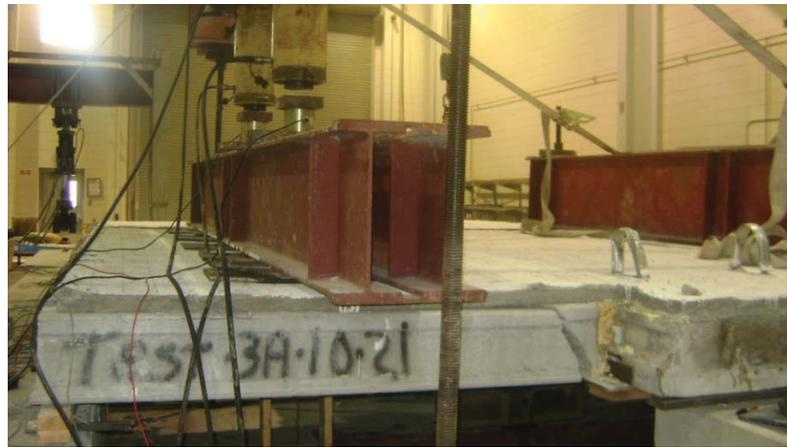
Figure 6.31: Failure of the HC at the critical section under ultimate loading
