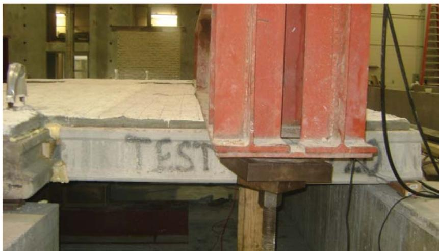
Figure 6.33: Failure of the HC at the critical section under ultimate loading
