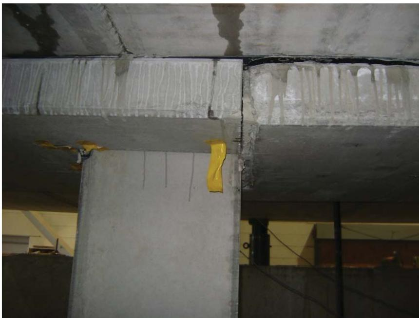
Figure 6.17: Failure of beam-column connection
