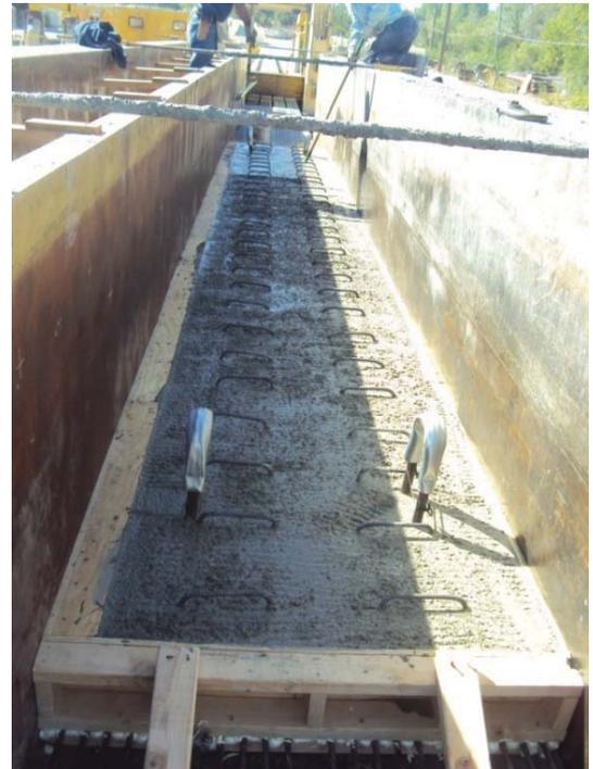
Fabrication of beam specimen
