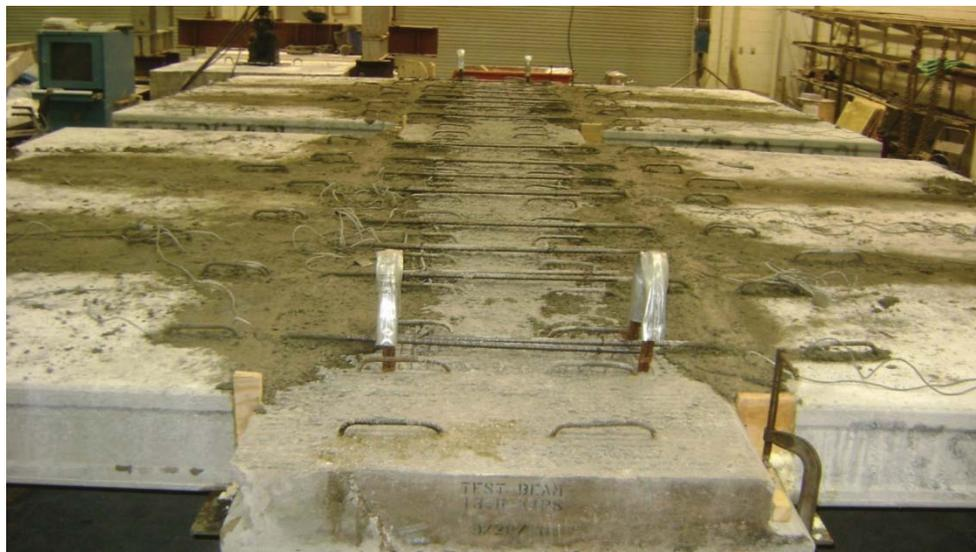
**Grouting hollow core key ways, HC opening and beam shear key**
