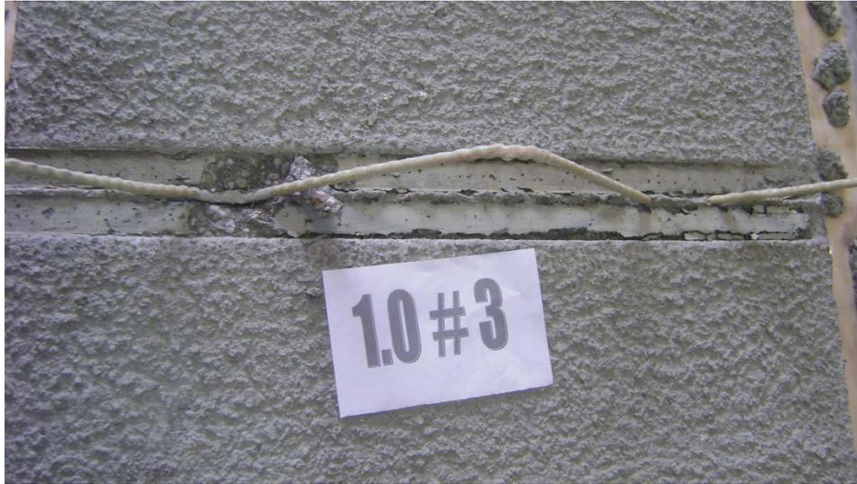
Figure 7.65: Pull-out of the tie from the concrete
