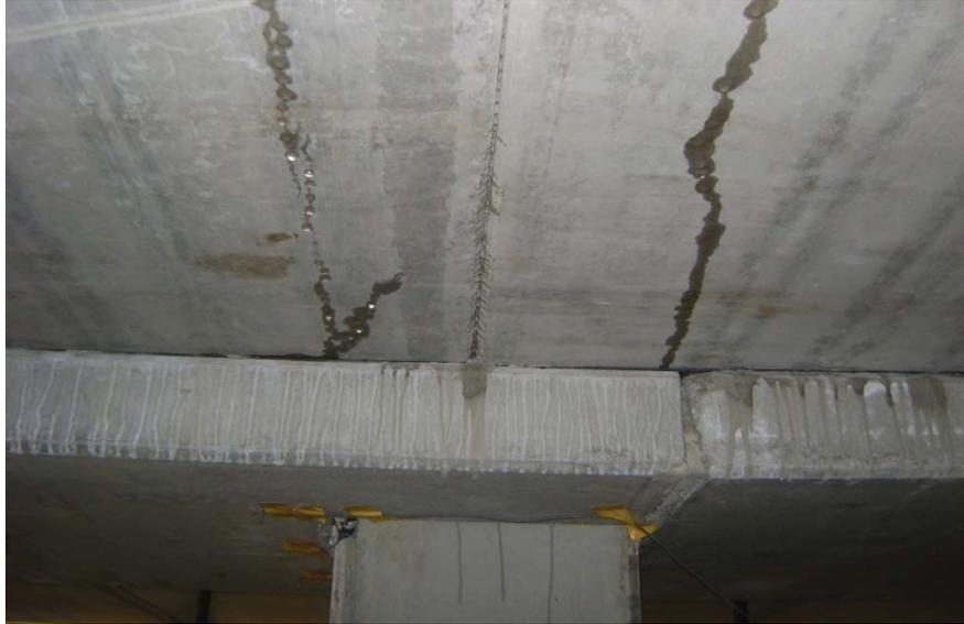
**Figure 6.14: Cracking of the HC soffit at ultimate load**
