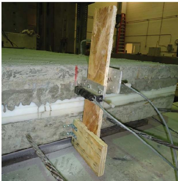
Figure 7.33: Measuring the relative movement between the bottom and top wythes
