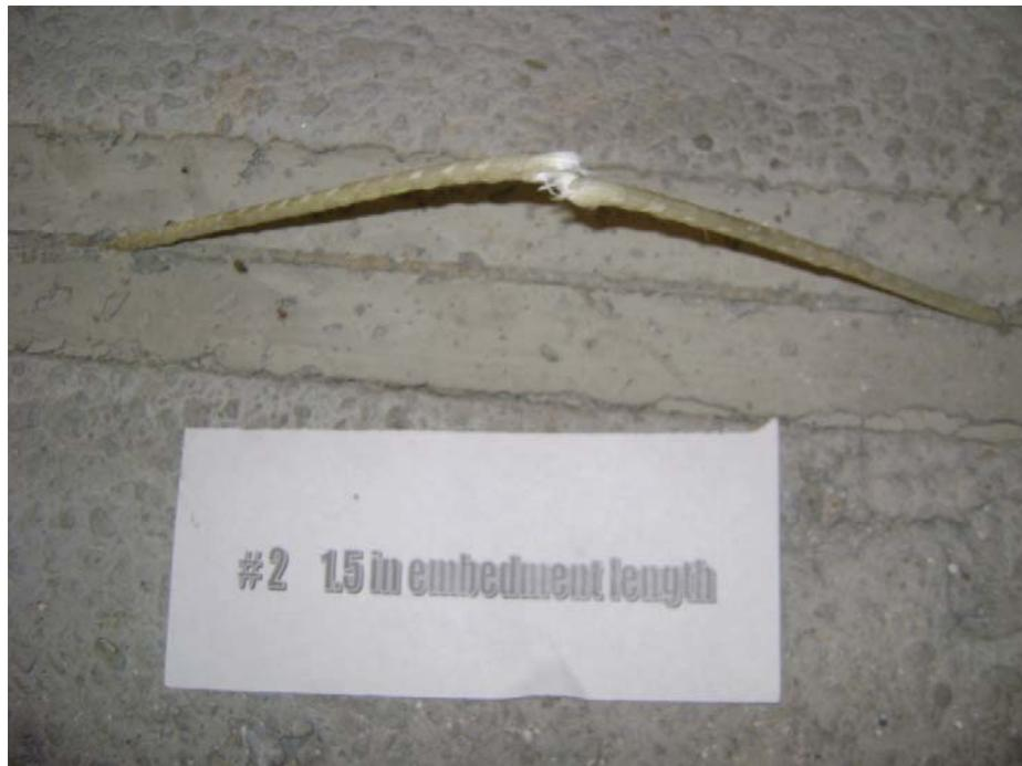
Figure 7.66: Rupture of the tie
