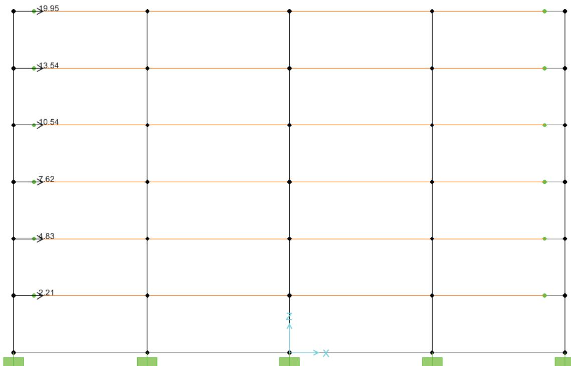
Figure 5.8: Seismic load applied to the beam direction
