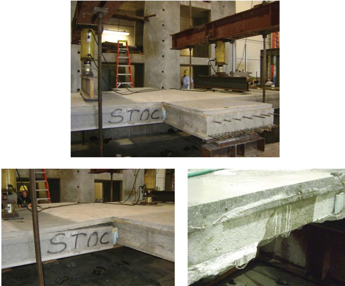
Figure 2.16: HC-beam connection under ultimate design load and failure of HC-beam connection. (Morcou and Tadros, 2010)
