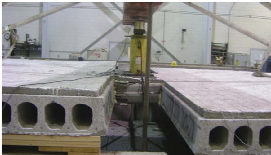
Figure 6.40: Failure mode of the flat soffit beam
