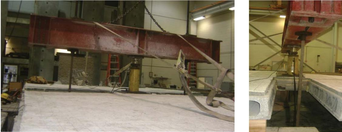
Figure 6.38: Flat soffit beam flexural test setup
