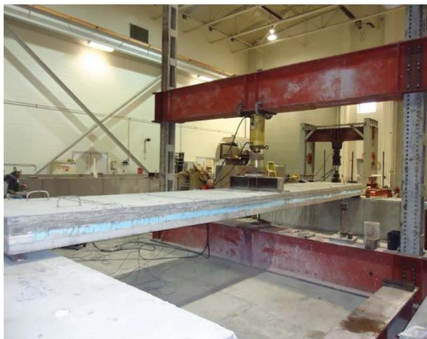
Figure 7.39: Test setup for panel D
