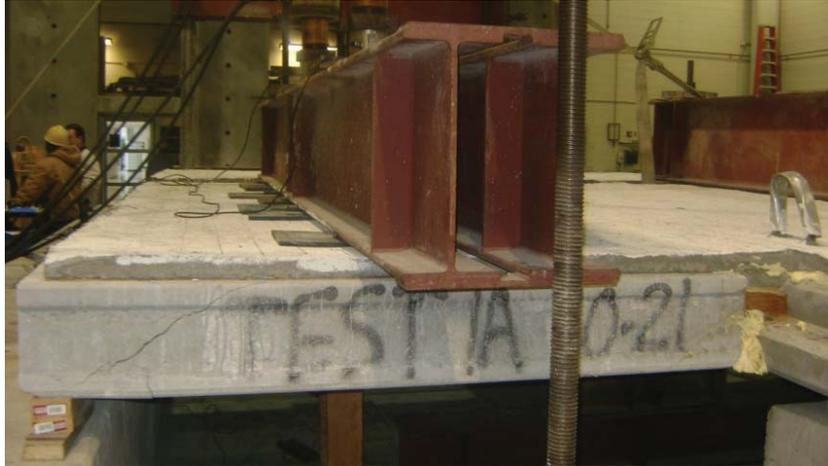
Figure 6.32: Failure of the HC at the critical section under ultimate loading
