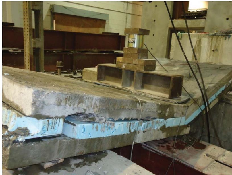
Figure 7.55: Shear failure of test 2 &3
