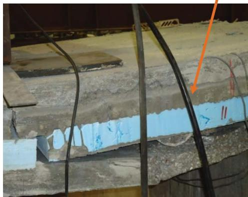
Figure 7.49: Shear failure of test 1
