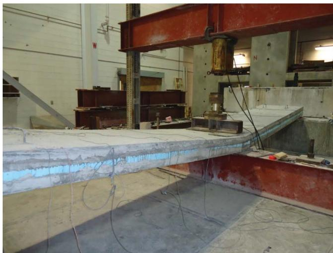
Figure 7.44: Failure mode of panel D
