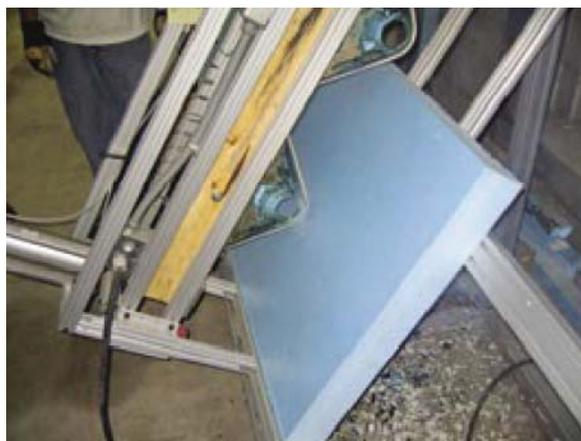
Figure 7.7: Hot melt slots into the foam blanks
