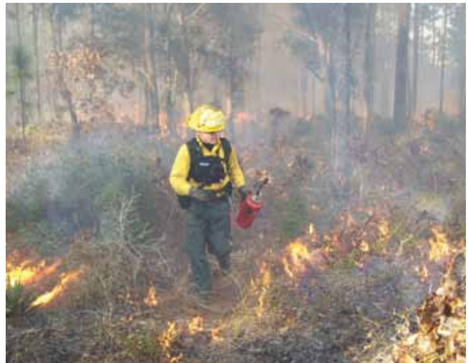
Matthew Dickinson helps with a January 2010 prescribed fire in longleaf pine-sandhill habitat at Eglin Air Force Base in Florida. Heat released by the fire was mapped by an airborne infrared camera calibrated by single-pixel infrared sensors mounted on 20-foot towers within the fire. Fuel consumption estimated from maps of total heat release will be compared with predictions from the model CONSUME.
