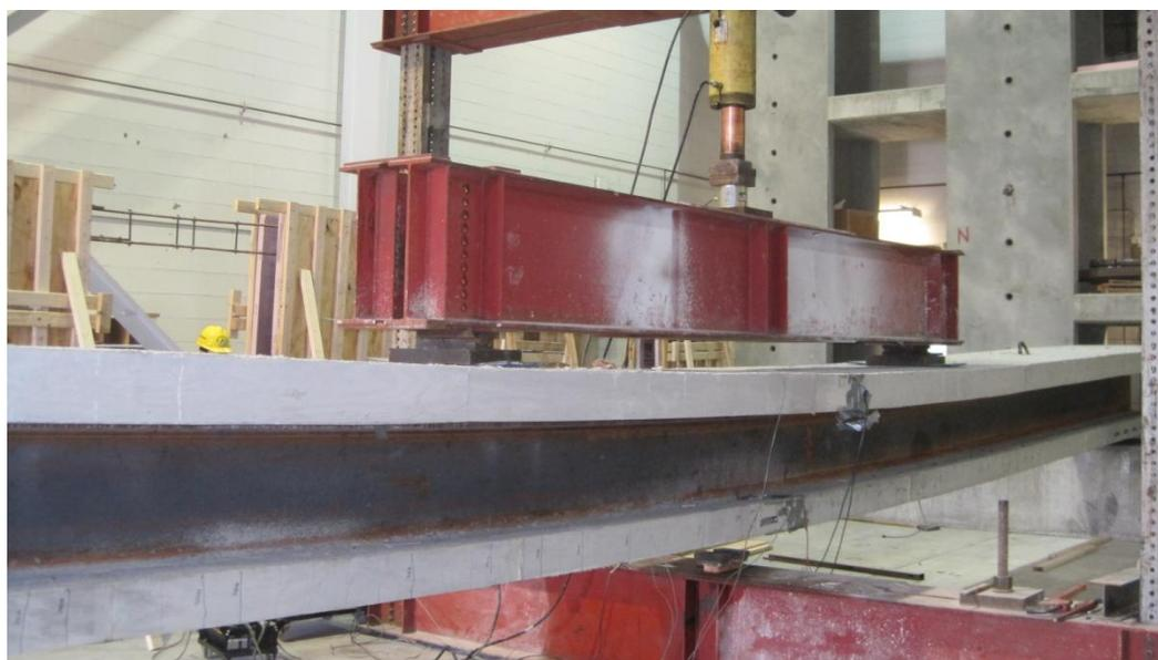
**Fig. 6.26 – Loading at Theoretical Ultimate Moment**
