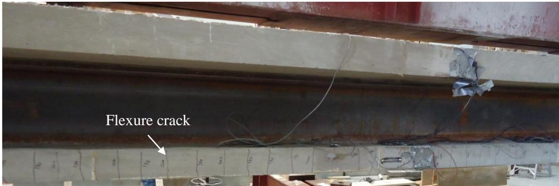
**Fig. 6.27 – Flexure Cracks in Flexural Test**
