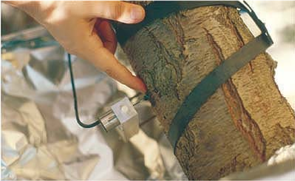
Figure 2.3. Linear variable differential transformer (LVDT; Goldhamer et al., 2003)
