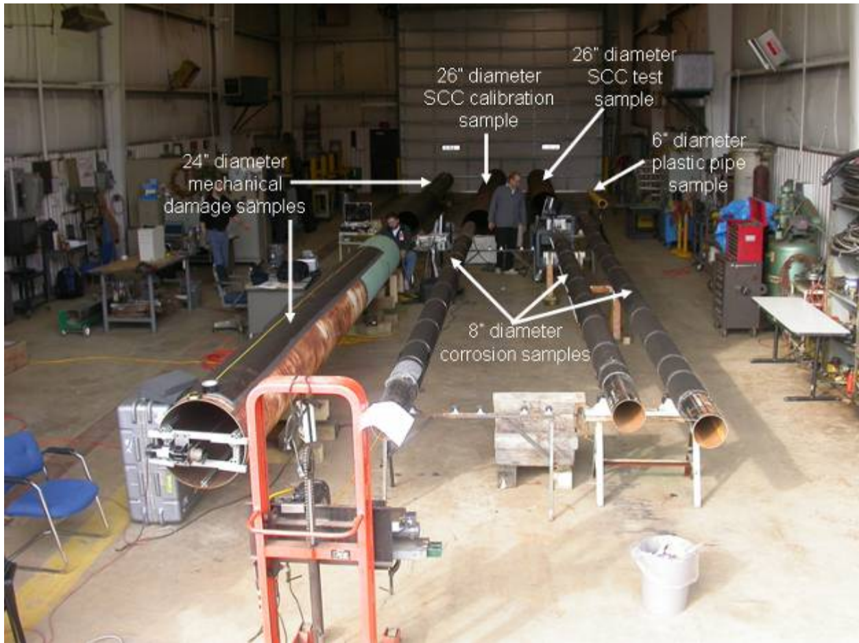
Figure 1-6. Benchmarking Demonstration Setup
