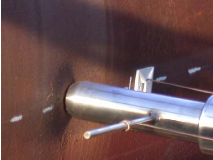
Figure 3-26. The spherical indenter, made from a non-ferromagnetic material, photographed while holding a 2 percent dent. Note the connections for the two linear cable extension transducers.
