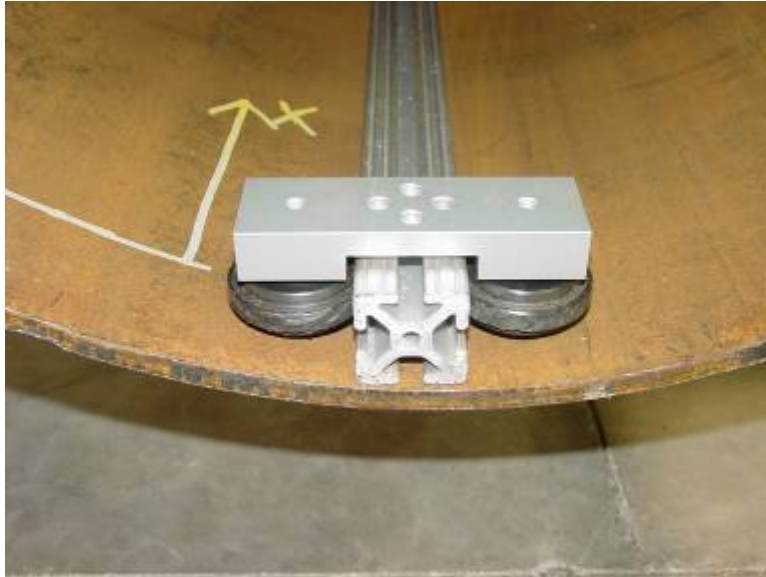
Figure 1-7. Aluminum Rail Guide Assembly
