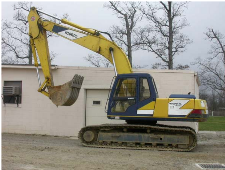
Figure 3-2. Kobelco Mark SK200 Track Hoe.
