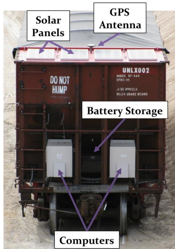
Figure 3-12. On-board computation, power supply, and GPS antenna.
