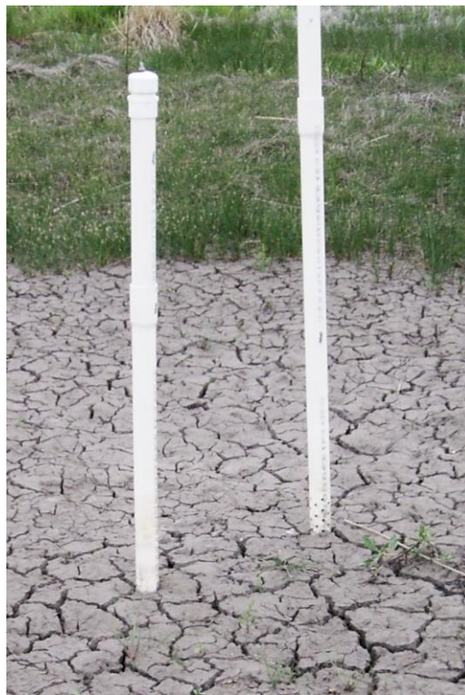
Figure 9: Example of an installed drive-point well (left) and stilling well (right).
