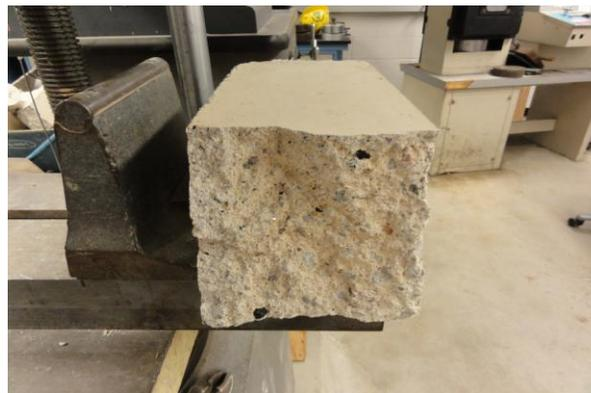
**Figure 3.2. Flexural Strength Testing for Experimental Concrete Mix**
