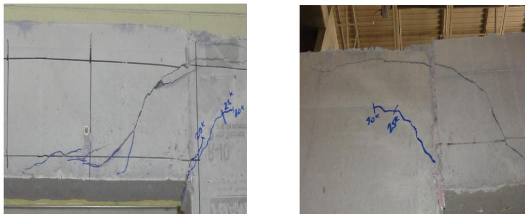
**Figure 3.15. Cracks Generation at Failure Load (Front and Back Side)**
