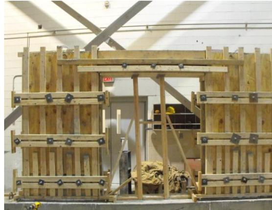
**Figure 3.32 Formwork Job Build ICF Wall**
