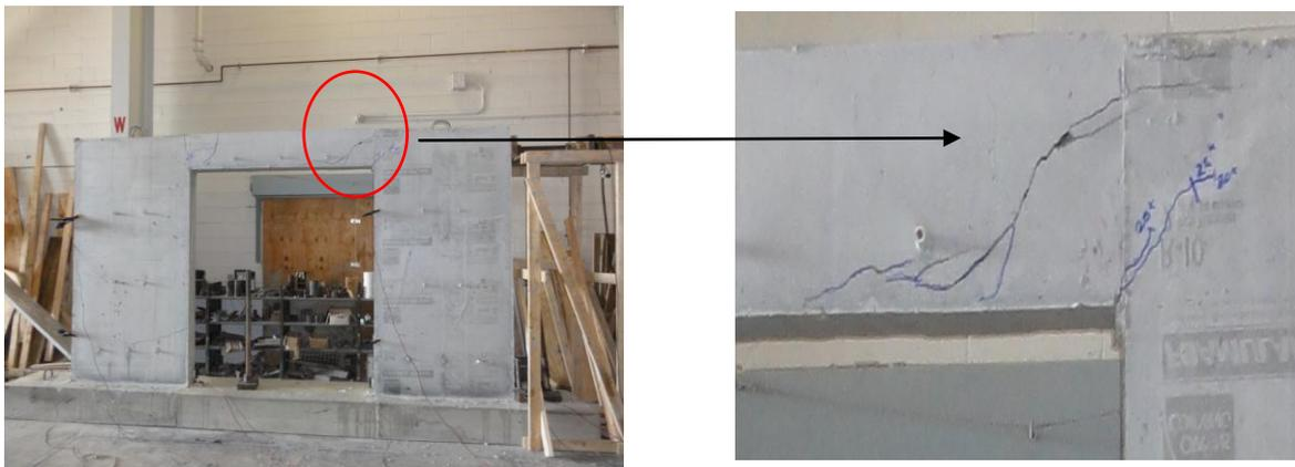
**Figure 3.3. Control Wall Structural Failure**
