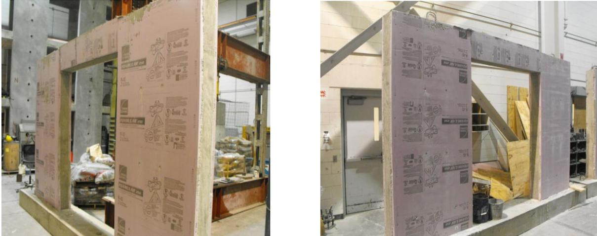
**Figure 2.9. Insulated Concrete Form Walls**
