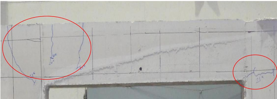
**Figure 3.28. Crack Generation at Load of 21,000lb (Front Side)**
