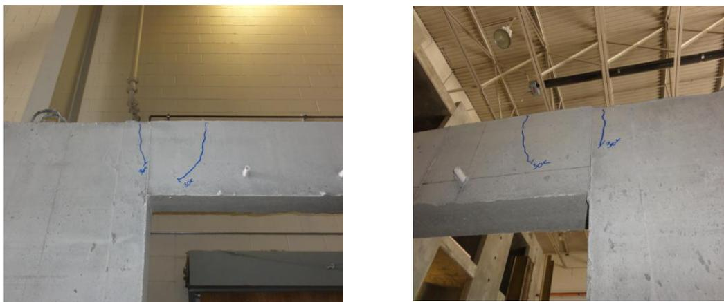
**Figure 3.14. Cracks Generation at Load of 30,000lb (Front and Back Side)**
