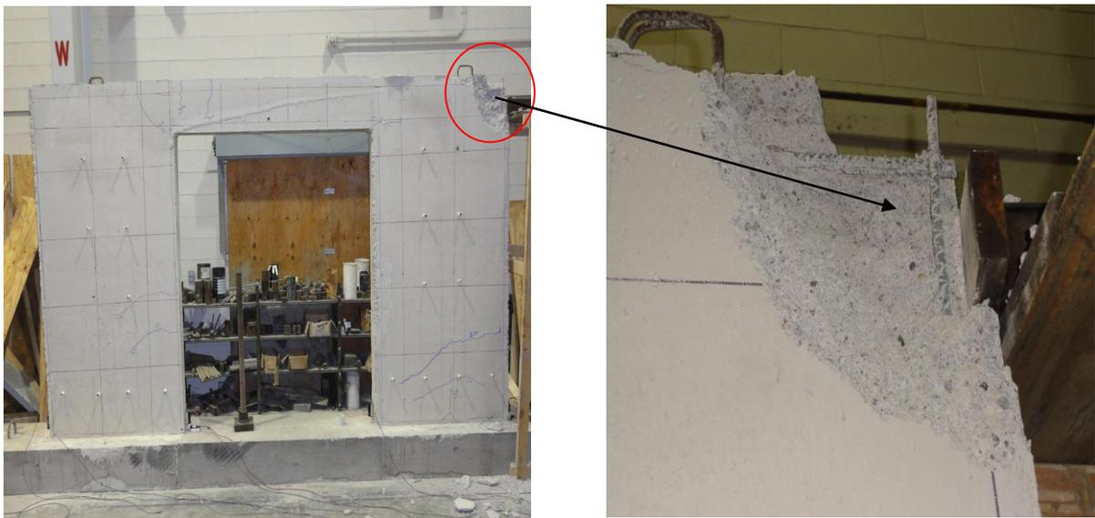
**Figure 3.30. Crack Generation at Failure Load (Front Side)**
