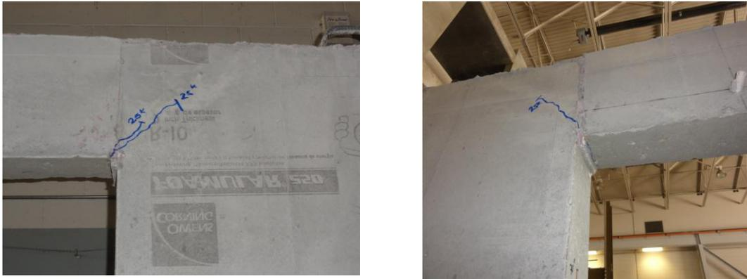
**Figure 3.13. Cracks Generation at Load of 25,000lb (Front and Back Side)**
