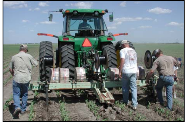
Spools of plastic subsurface irrigation line, or drip tape, are buried about a foot below the surface of this field at UNL's South Central Agricultural laboratory near Clay Center (photo: Suat Irmak).
