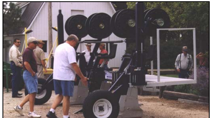
Examining equipment used to install subsurface drip irrigation lines at a Kansas State University subsurface drip irrigation field day in Colby, KS in July (photo: Steve Ress).
