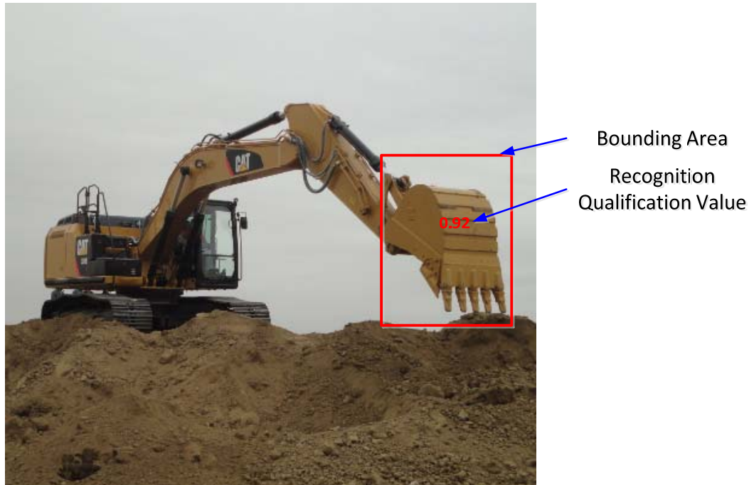
Figure 8. Recognition and tracking heavy equipment's dynamic component by a digital camera
