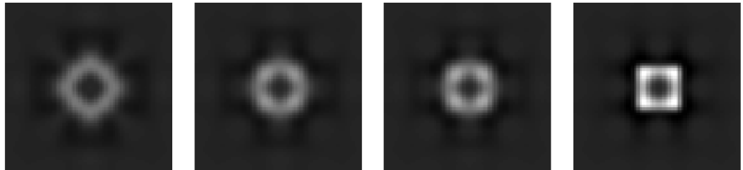
B. Differences with Wiener transfer function, left-to-right: optimal 2D PCC, optimal separable PCC, separable PCC ( \alpha = -0.5 ), cubic spline interpolation
