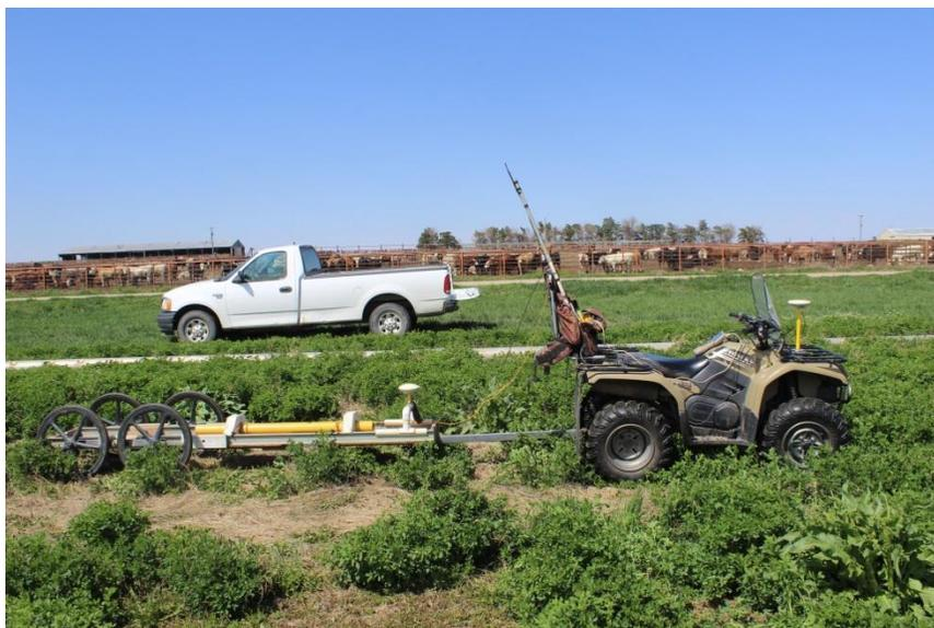
**Figure B.4 Apparent Electrical Conductivity Apparatus used to Determine Manure Accumulation Patterns on Both Fields**
