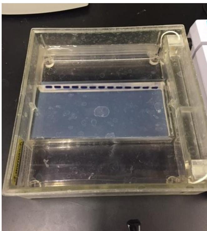
**Figure B.10 Gel Electrophoresis Apparatus**
