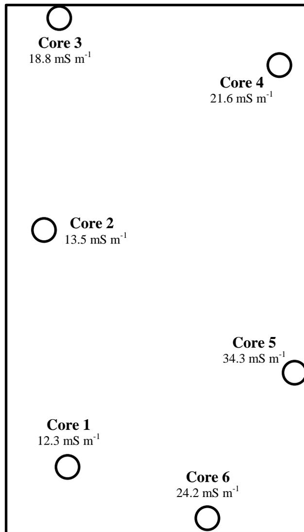
**Figure 2.3 Schematic of Sampling Locations and Electrical Conductivity Measurements**
