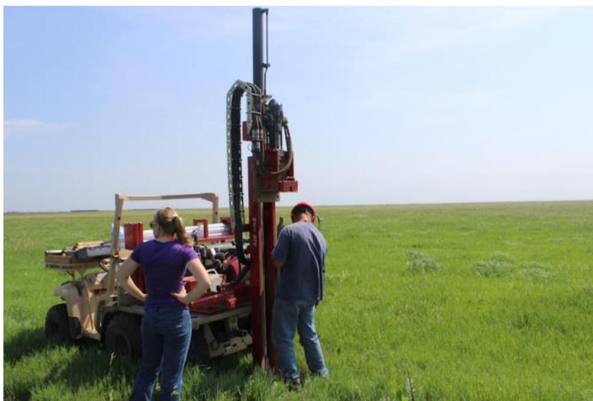
**Figure B.5 Hydraulic Soil Probe used to Extract Intact Soil Cores**
