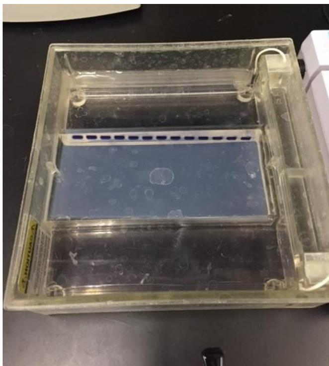
**Figure B.10 Gel Electrophoresis Apparatus**
