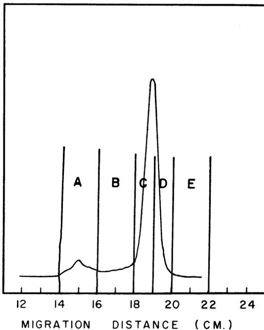
FIG. 2. Electrophoretic diagram of thermal aldolase. Conditions were: diethylbarbiturate buffer (pH 8.6), ionic strength, 0.075; 18 hr at 180 VDC. Segments (A, B, C, D, and E) were cut from strip and assayed for aldolase. The moles of triose formed  $\times 10^{-8}$  were as follows for each segment: A (origin), 0; B, 0.5; C, 12.5; D, 8.3; E, 0.
