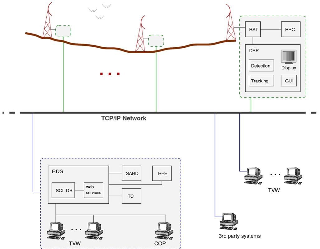
Figure 1: Desired 3D Avian Radar Systems Design
