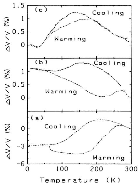
FIG. 2. (a) Temperature dependence of the longitudinal wave velocity with  $\hat{q} \parallel c$  in zero field at 12 MHz. (b) Shear wave velocity for  $f=14.5$  MHz with  $\hat{q} \parallel c$  in zero field. (c) Longitudinal wave velocity with  $\hat{q} \parallel$ (basal plane) in zero field at 12.0 MHz.
