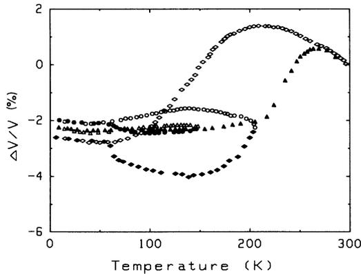
FIG. 3. Thermal hysteresis behavior of the longitudinal wave velocity with  $\hat{q}\parallel c$  in zero field at 12 MHz. The point designations and the order of the temperature steps are as follows: cooling down from room temperature to 4 K ( $\diamond$ ); warming from 4 to 200 K ( $\blacklozenge$ ); cooling from 200 to 4 K ( $\circ$ ); warming from 4 to 145 K ( $\bullet$ ); cooling from 145 to 4 K ( $\triangle$ ); and warming from 4 K to room temperature ( $\blacktriangle$ ).
