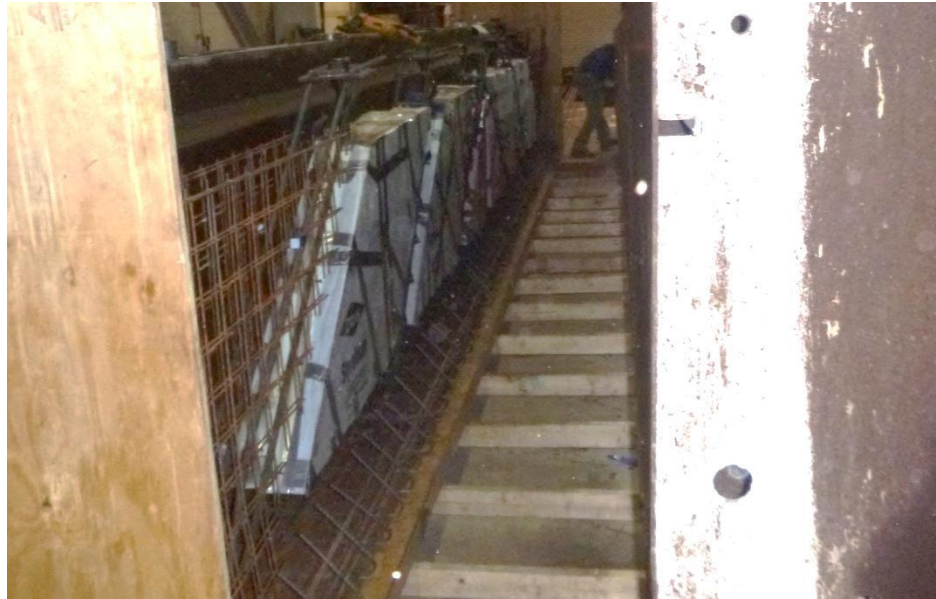
Figure 4.24 Full span of the specimen before closing the form
