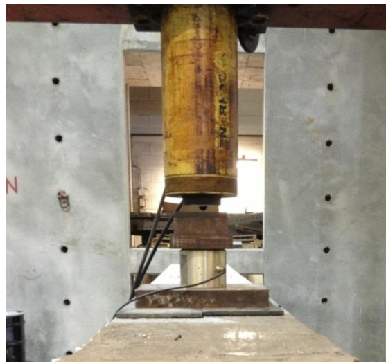
Figure 4.42 The plates' organization and the load cell at the point of loading
