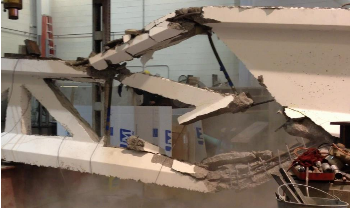
Figure 4.50 The moment of failure of the truss
