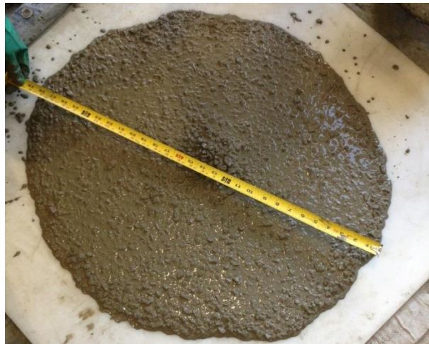
Figure 4.27 Self-consolidating concrete spread test
