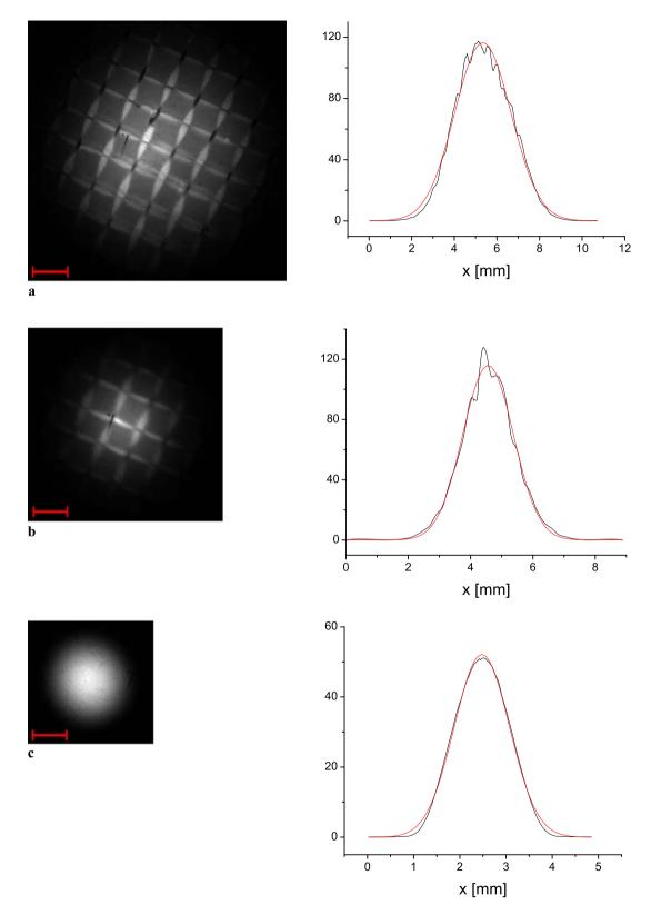
Fig. 3 Beam patterns and profiles with the mesh anode in place. Line outs and Gaussian fits are shown. The *red bars* indicate a distance of 1 mm on the detector. **a** Beam pattern and profile for illumination of cathode with fundamental; **b** with second harmonic; **c** with third harmonic light
