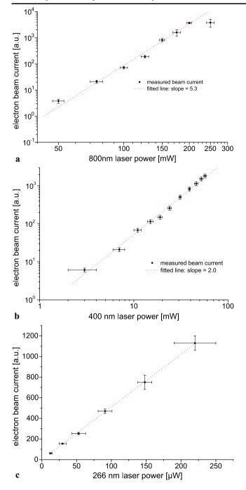
Fig. 2 a Electron beam current vs. fundamental laser power. The data are fitted with a power law with slope 5.3 indicating above threshold emission. **b** Electron beam current vs. laser power for 400-nm laser light (second harmonic). A power law with a power of two describes the dependence. **c** Electron beam current vs. third harmonic laser power. A linear correlation is obtained
