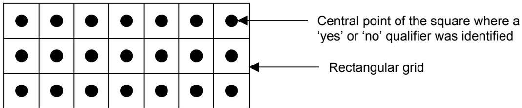
Figure 3. Top view of tank surface illustrating grid method used to assess intactness of the rubber cover
