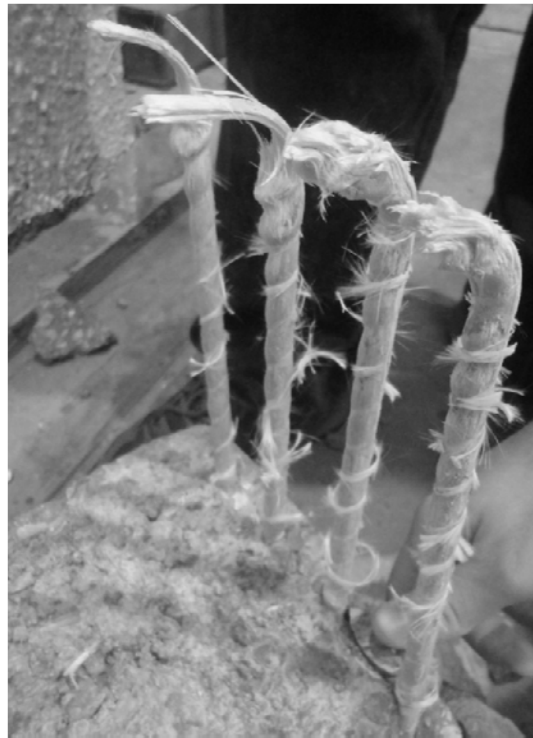
Figure 4-12: Ruptured GFRP Bars in specimen B1
