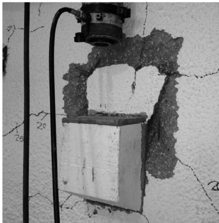
Figure 4-8: Specimen A1 crack pattern at failure
