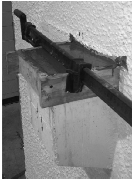
Figure 4-6: Forming of leveling grout pad used for specimens A1, A2 and B1
