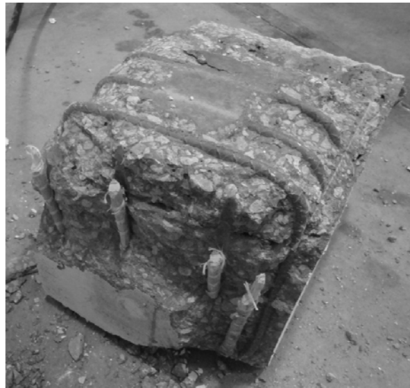
Figure 4-15: Marked Cracks at failure and failure mode of specimen B2
