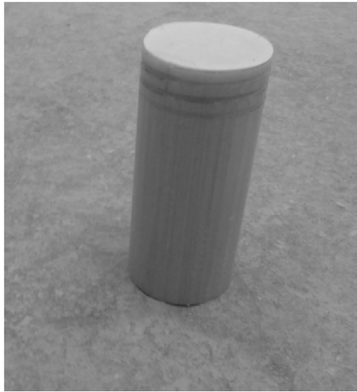
Figure 3-22: GFRP Pin 2" diameter x 4½" long
