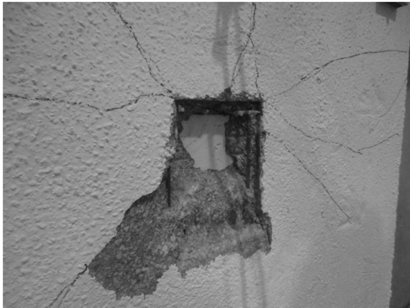
Figure 4-15: Marked Cracks at failure and failure mode of specimen B2
