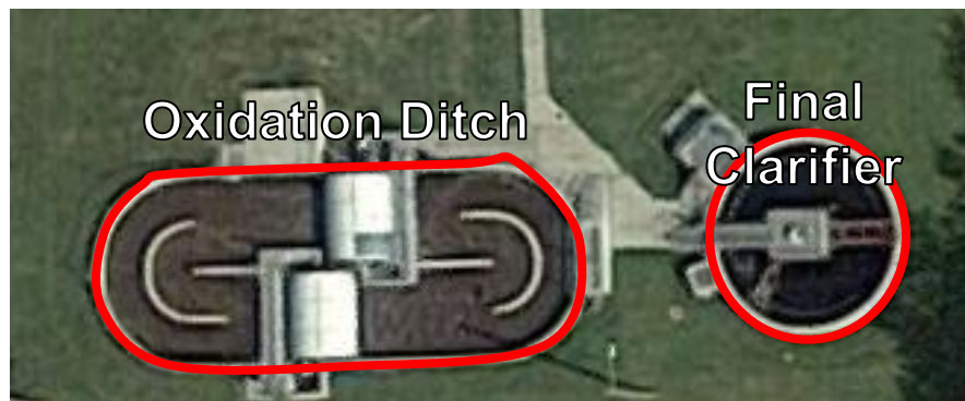
Figure 2.4: Aerial View of a Small Oxidation Ditch Plant (Google Maps, 2017b).
