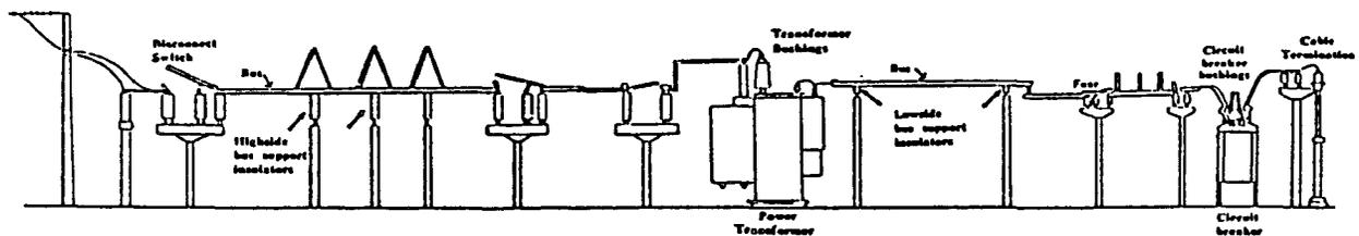
Figure 1. Simplified schematic of a substation showing some of the equipment most commonly experiencing animal-caused faults.
