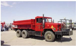
This 2 ½ ton 6x6 tanker was supplied by NFS to a fire department through the Federal Excess Property Program. The Fire Shop made repairs and brought the tanker up to safety standards and the cooperating fire department (Dannebrog) did the finish work on the vehicle.
