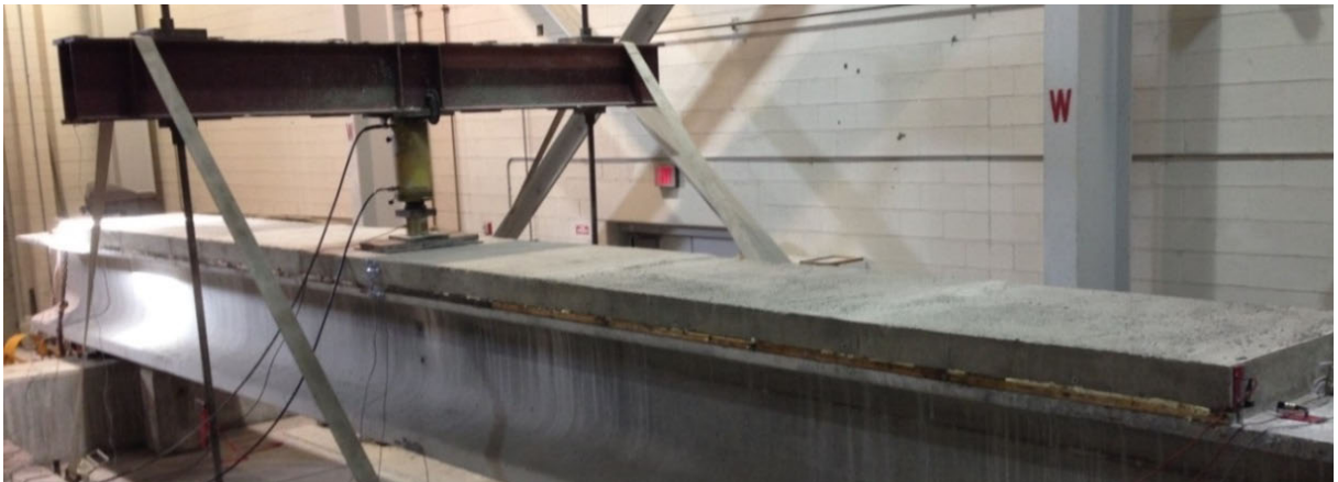
FIGURE 6-32: TEST SETUP ON FULL FLANGE GIRDER
