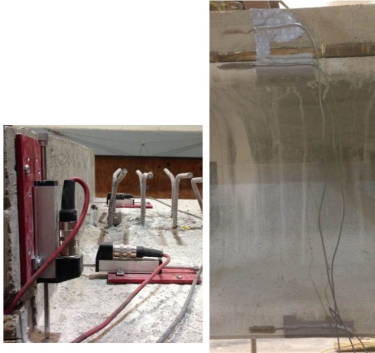
FIGURE 6-31: LVDT'S (LEFT), STRAIN GAUGES (RIGHT)
