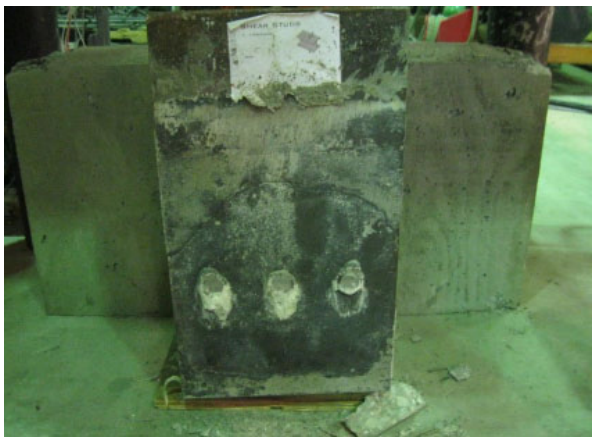
FIGURE 2-5: SHEAR STUD CONNECTOR FAILURE MODE (COURTESY OF ISU BRIDGE CENTER)
