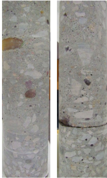
FIGURE 6-3: CORES TAKEN FROM BONDED ZONE (LEFT) AND FROM DEBONDED ZONE (RIGHT)
