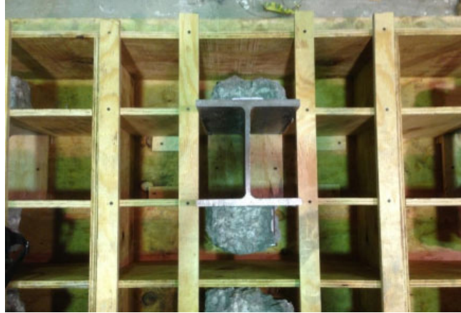
FIGURE 2-3: SPECIMEN FORMING ( COURTESY OF ISU BRIDGE CENTER )
