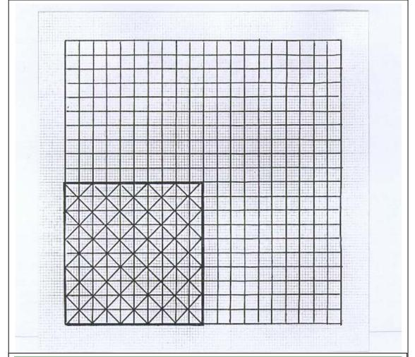
20 x 20 cm square grid for sorting total defects from sound whole sorghum grains, with a 10 x 10 cm insert for checking sample size
