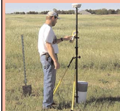
Facilities Operations performs surveying using an RTK (Real Time Kinematics) GPS (Global Positioning System). This system allows Facilities Operations locate infrastructure at the ARDC to within less than one half inch. This system is used to collect GIS (Geographical Information Systems) data for use by other departments.
