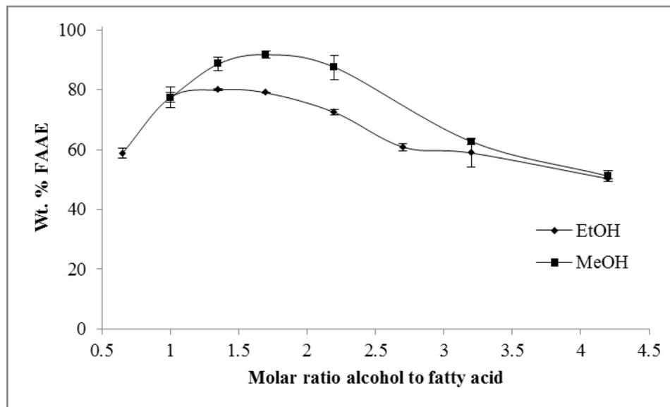
Figure 3.3 Effect of ethanol level on the esterification of FFA to FAEE with 0.71 g immobilized CalB, 8 g oleic acid, 0.9 g water, 50 °C, and 3 h.
