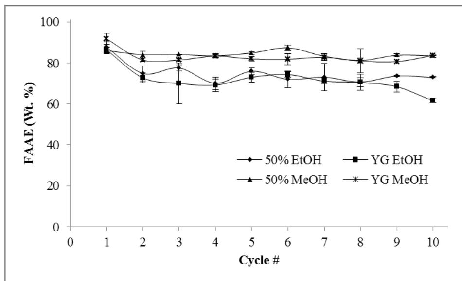
Figure 3.10 Reuse of both immobilized lipase PS and immobilized CalB in the esterification and transesterification of a 50% FFA substrate and yellow grease to FFAE at 8 g combined soybean oil and oleic acid or yellow grease, 1.54 g immobilized lipase PS, 1.43 g immobilized CalB, 1.74 g ethanol, 0.9 g water, 50 °C, and 6 h, and compared to the same reactions using methanol.
