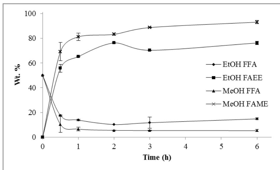
Figure 3.7 Comparison of methanol and ethanol as acyl acceptor with combined lipases and at respective optimized conditions on a 50% FFA model substrate.
