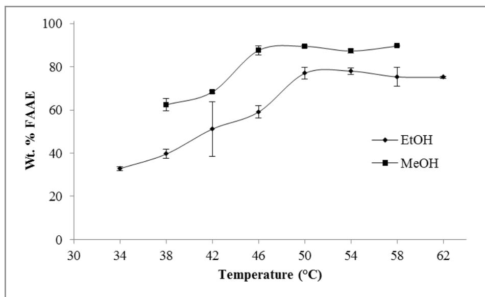
Figure 3.1 Effect of temperature on the esterification of FFA to FAEE with 0.71 g immobilized CalB, 8 g oleic acid, 2.22 g ethanol, 0.36 g water, and 3 h.
