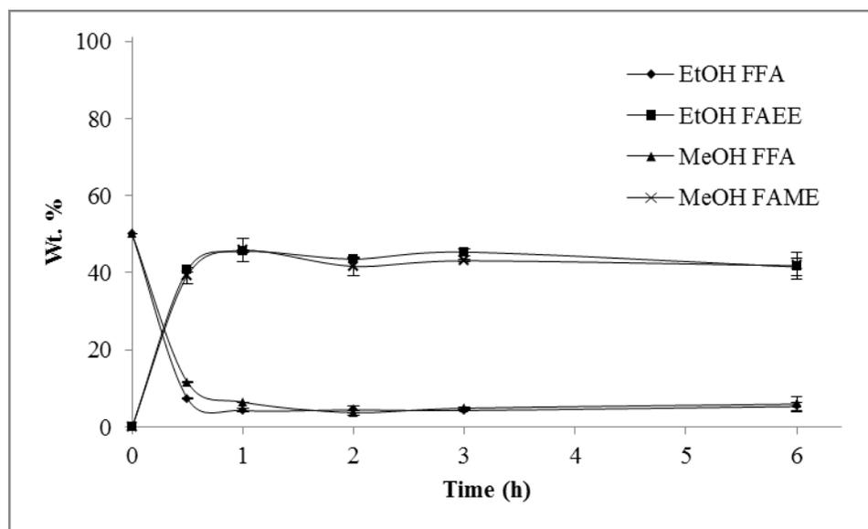
Figure 3.4 Esterification and transesterification of FFA and triglycerides to FAEE using immobilized CalB at the optimized conditions on a 50% FFA substrate at 4 g oleic acid, 4 g soybean oil, 1.54 g immobilized lipase PS or 1.43 g immobilized CalB, 1.74 g ethanol, 0.9 g water, and 50 °C.
