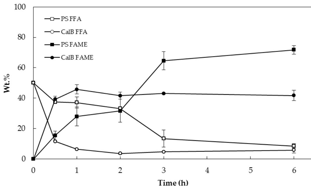
Figure 2.4 Esterification and transesterification of FFA and triglycerides to FAME using immobilized lipase PS and CalB separately at the optimized conditions on a 50% FFA substrate at 4 g oleic acid, 4 g soybean oil, 1.54 g immobilized lipase PS or 1.43 g immobilized CalB, 1.54 g methanol, 0.36 g water, and 50 °C.
