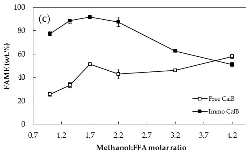
Figure 2.3 Effect of methanol:FFA molar ratio on FFA esterification to FAME at 30 mg free CalB or 0.71 g immobilized CalB, 8 g oleic acid, 0.36 g water, 50 °C, and 3 h.
