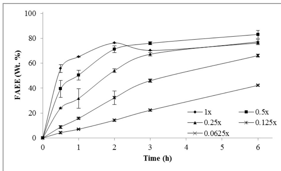
Figure 3.9 Effect of varied enzyme loading on esterification and transesterification of FFA and triglycerides to FAEE with both immobilized lipase PS and immobilized CalB on a 50% FFA substrate, with FAEE plotted against time, at 4 g oleic acid, 4 g soybean oil, 1.74 g ethanol, 0.9 g water, and 50 °C.
