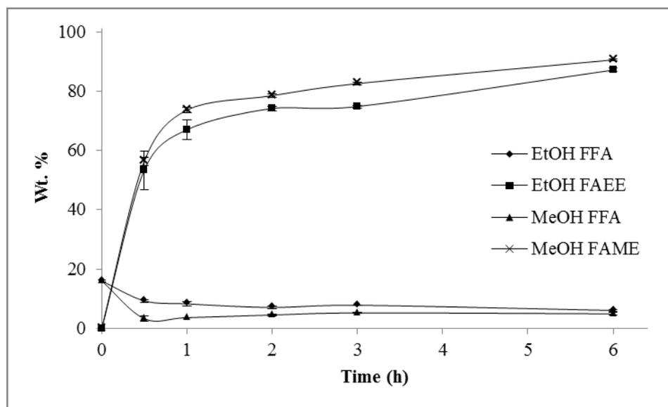
Figure 3.8 Comparison of methanol and ethanol as acyl acceptor with combined lipases and at respective optimized conditions on yellow grease.
