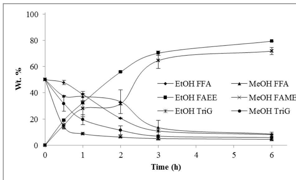
Figure 3.5 Esterification and transesterification of FFA and triglycerides to FAEE using immobilized lipase PS at the optimized conditions on a 50% FFA substrate at 4 g oleic acid, 4 g soybean oil, 1.54 g immobilized lipase PS or 1.43 g immobilized CalB, 1.74 g ethanol, 0.9 g water, and 50 °C.
