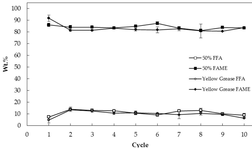
Figure 2.8 Reuse of both immobilized lipase PS and immobilized CalB in the esterification and transesterification of a 50% FFA substrate and yellow grease to FAME at 8 g combined soybean oil and oleic acid or yellow grease, 1.54 g immobilized lipase PS, 1.43 g immobilized CalB, 1.54 g methanol, 0.36 g water, 50 °C, and 6 h.
