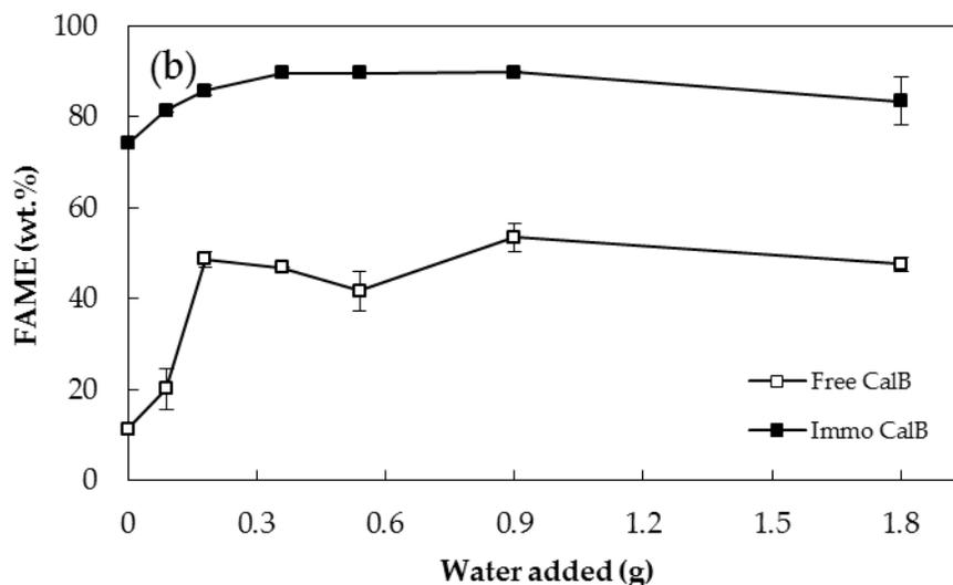
Figure 2.2 Effect of water level on FFA esterification to FAME at 30 mg free CalB or 0.71 g immobilized CalB, 8 g oleic acid, 1.36 g methanol, 50 °C, and 3 h.
