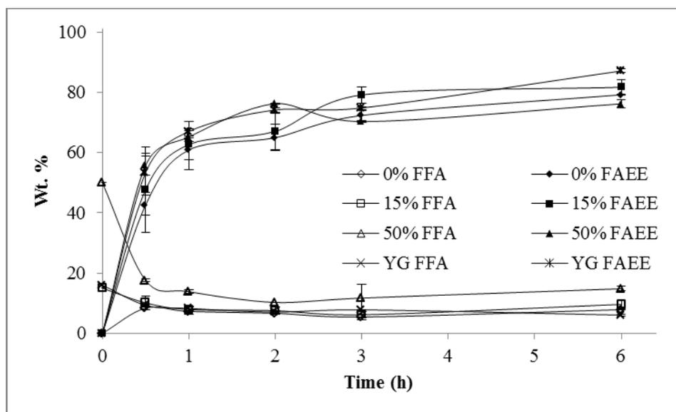
Figure 3.6 Esterification and transesterification of FFA and triglycerides to FAEE using immobilized lipase PS and immobilized CalB together in a single reaction on substrates with varied initial FFA wt.% and yellow grease at 8 g combined soybean oil and oleic acid or yellow grease, 1.54 g immobilized lipase PS, 1.43 g immobilized CalB, 1.74 g ethanol, 0.9 g water, and 50 °C.
