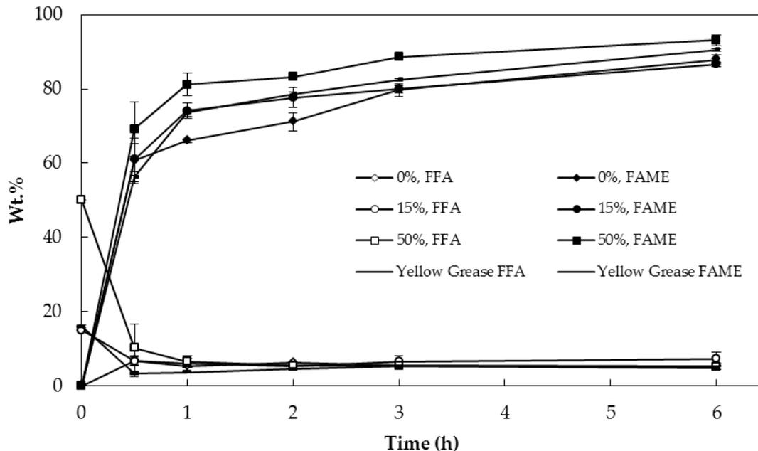
Figure 2.5 Esterification and transesterification of FFA and triglycerides to FAME using immobilized lipase PS and immobilized CalB together in a single reaction on substrates with varied initial FFA wt.% and yellow grease at 8 g combined soybean oil and oleic acid or yellow grease, 1.54 g immobilized lipase PS, 1.43 g immobilized CalB, 1.54 g methanol, 0.36 g water, and 50 °C.
