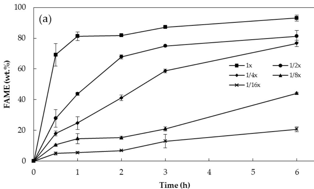
Figure 2.6 Effect of varied enzyme loading on esterification and transesterification of FFA and triglycerides to FAME with both immobilized lipase PS and immobilized CalB on a 50% FFA substrate : FAME production with time. All reactions at 4 g oleic acid, 4 g soybean oil, 1.54 g methanol, 0.36 g water, and 50 °C.
