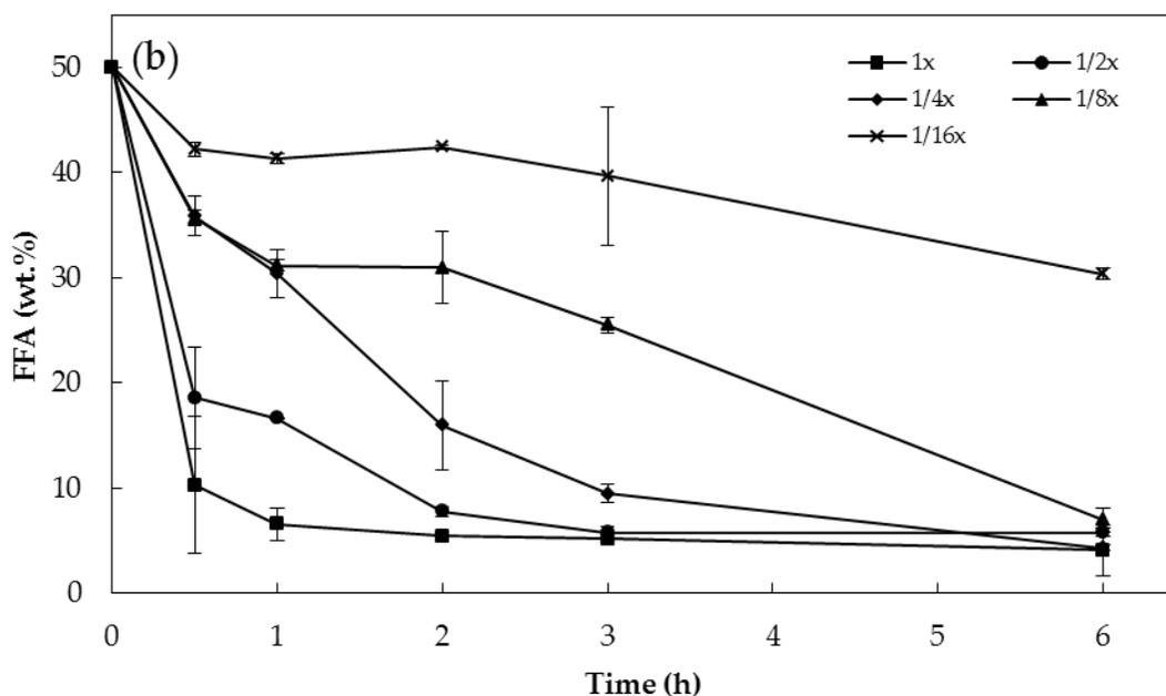
Figure 2.7 Effect of varied enzyme loading on esterification and transesterification of FFA and triglycerides to FAME with both immobilized lipase PS and immobilized CalB on a 50% FFA substrate. All reactions at 4 g oleic acid, 4 g soybean oil, 1.54 g methanol, 0.36 g water, and 50 °C.
