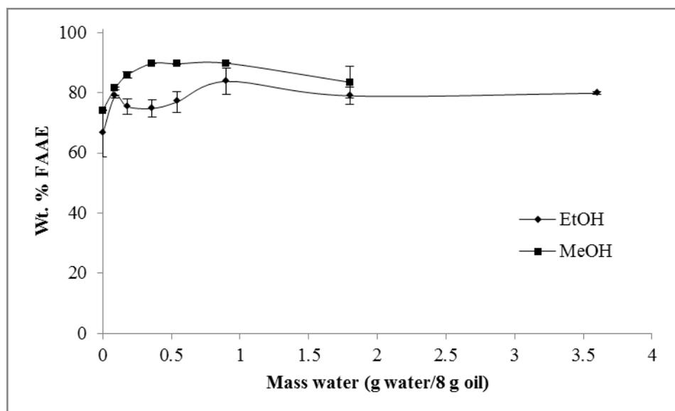
Figure 3.2 Effect of water on the esterification of FFA to FAEE with 0.71 g immobilized CalB, 8 g oleic acid, 2.22 g ethanol, 50 °C, and 3 h.
