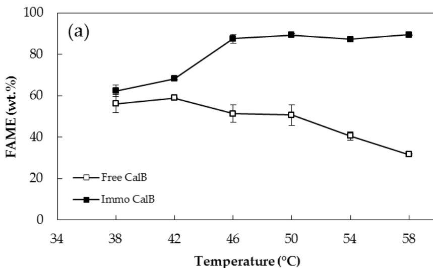
Figure 2.1 Effect of reaction temperature on FFA esterification to FAME at 30 mg free CalB or 0.71 g immobilized CalB, 8 g oleic acid, 1.36 g methanol, 0.2 g water, and 3 h.
