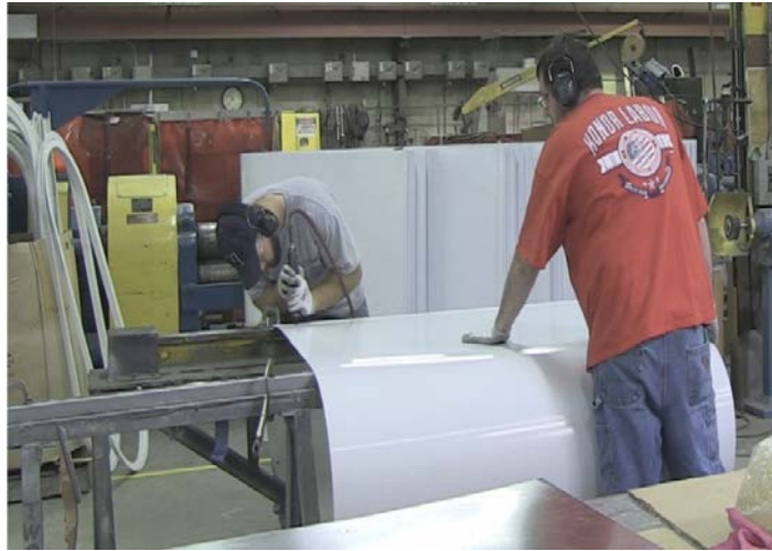
Figure 5.4: Lock Setting Task Performed By Crew 2
