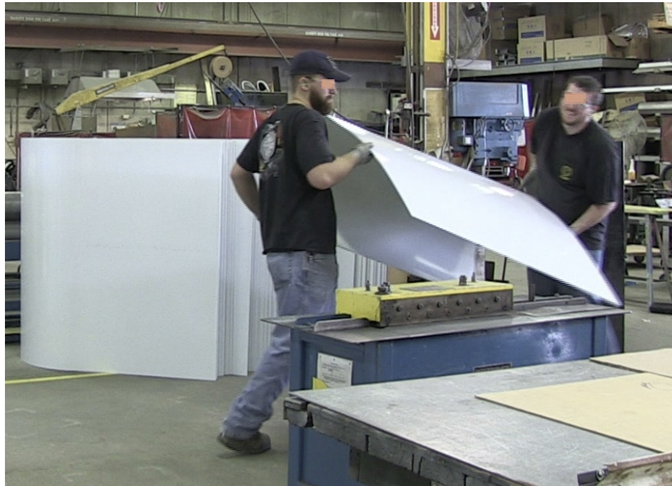
Figure B.3: Move the Roll-Bended Sheet to the Lock Forming Table (M 3 )
