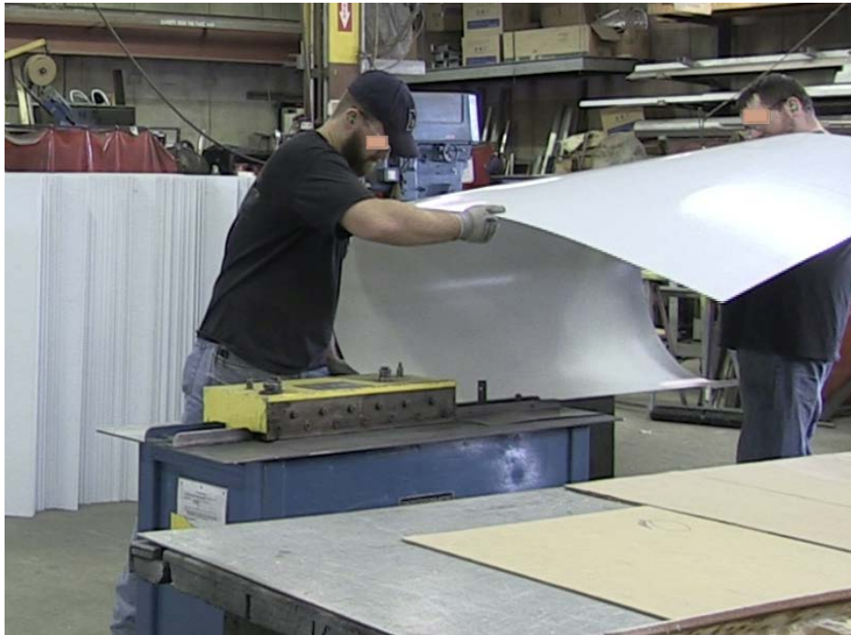
Figure B.5: Set One Edge of the Roll-Bended Sheet on Lock Machine (M 5 )
