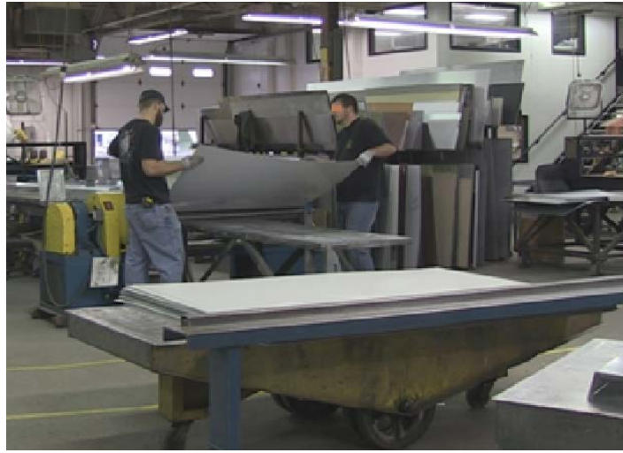
Figure 5.2: Roll Bending Task Performed By Crew 2
