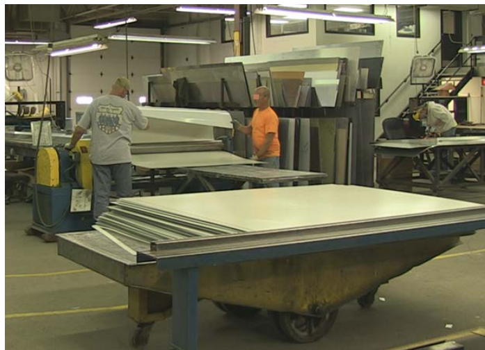
Figure 5.1: Roll Bending Task Performed By Crew 1
