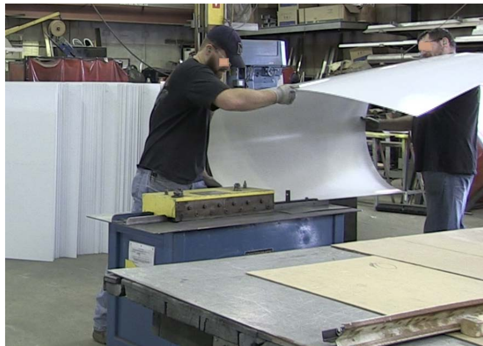
Figure B.4: Place the Roll-Bended Sheet on the Lock Forming Table (M 4 )
