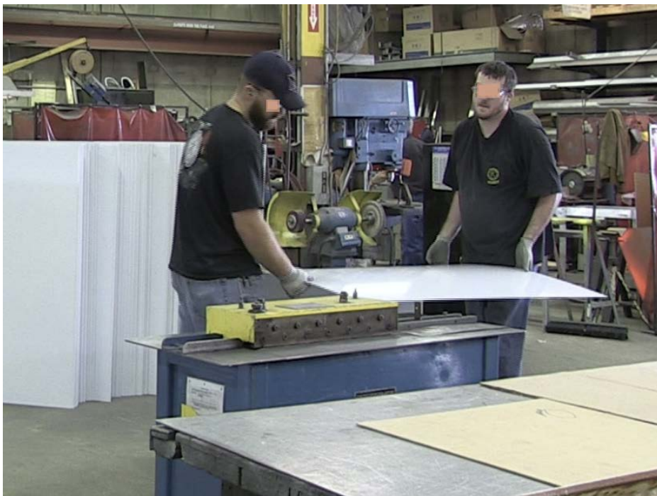
Figure B.8: Place Another Edge of the Sheet on Lock Machine (M 8 )
