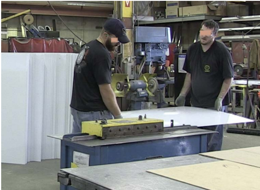
Figure B.9: Set Another Edge of the Sheet on Lock Machine (M 9 )
