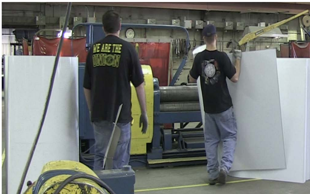
Figure B.13: Place the Lock Formed Sheet at Stacks (M 13 )
