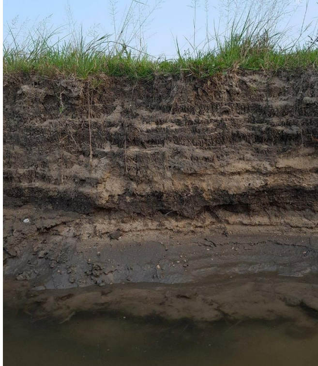
Figure 2.2 Typical streambank on Cedar River. Note the transition from sandy soil at the top to silty loam in the bottom.
