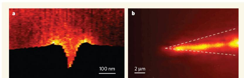
Figure 2. Into the groove. **a**, Ropers and colleagues' 'tip-enhanced electron emission microscopy'<sup>1</sup> provides a picture of a nanoscale groove in a gold surface. **b**, The laser-illuminated probe tip.
