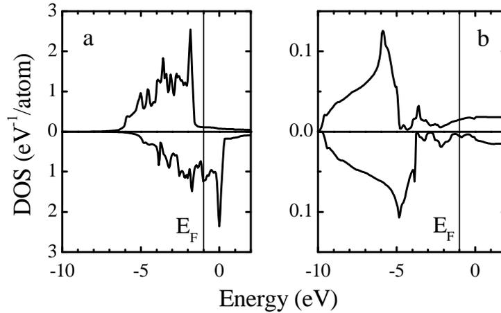
**Fig.13** Density of states for bulk fcc Co projected to the d orbitals (a) and the s orbitals (b) for the majority-spin electrons (top panels) and minority-spin electrons (bottom panels). The spin polarization of the d-DOS at the Fermi energy is opposite to that for the s-DOS. Note a different scale in (a) and (b).
