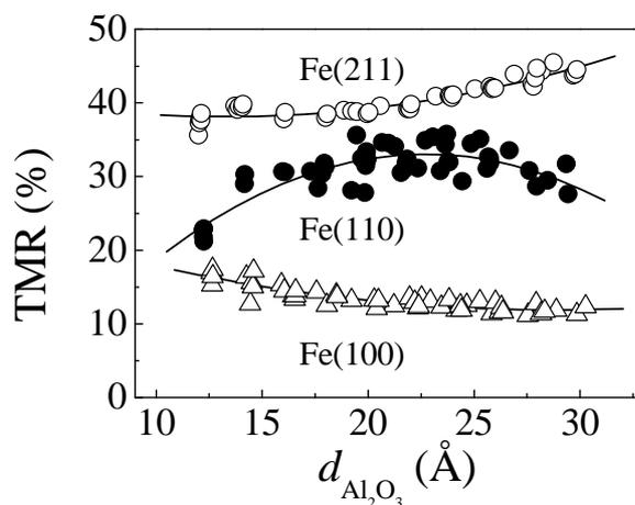
**Fig.9** TMR at 2K as a function of Al<sub>2</sub>O<sub>3</sub> thickness for Fe(211), Fe(110), and Fe(100) epitaxial electrodes in Fe/Al<sub>2</sub>O<sub>3</sub>/CoFe junctions. Lines are only a guide to the eye. From Yuasa *et al.* [67].
