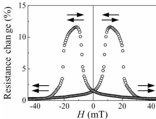
**Fig.1** First observation of reproducible, large room temperature magnetoresistance in a  $\text{CoFe}/\text{Al}_2\text{O}_3/\text{Co}$  magnetic tunnel junction. The arrows indicate the relative magnetization orientation in the CoFe and Co layers. After Moodera *et al.* [3].
