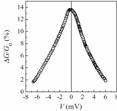
**Fig.4** Original demonstration of the tunneling magnetoresistance effect. The relative conductance change due to an applied magnetic field versus applied bias in a Fe/Ge/Co junction at 4.2 K. After Julliere [1].
