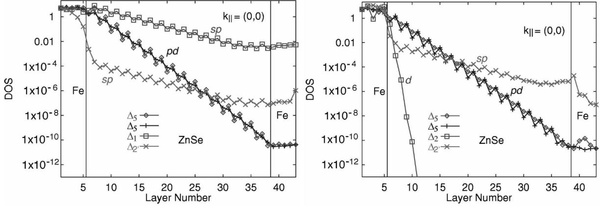
**Fig.15** The calculated layer-dependent density of states (DOS) for the majority (a) and minority (b) Bloch states at  $\mathbf{k}_{\parallel}=0$  for Fe/ZnSe/Fe junction. Different decay rates and injection efficiencies for the states of different character and symmetry are seen. After MacLaren *et al.* [128].
