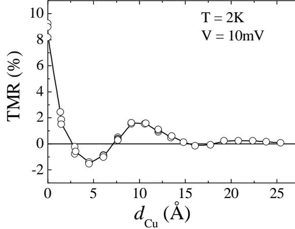
**Fig.12** TMR at 2K and a bias of 10mV as a function of Cu interlayer thickness for Co(001)/Cu(001)/Al<sub>2</sub>O<sub>3</sub>/Ni<sub>80</sub>Fe<sub>20</sub> junctions. The period of the oscillation observed, 11.4Å, is in agreement with the Fermi surface of Cu. From Yuasa *et al.* [103].
