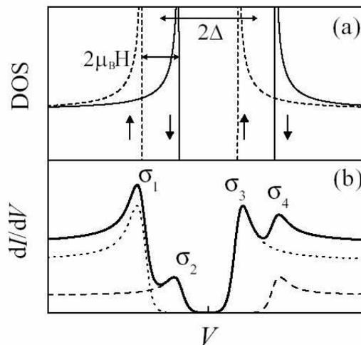
**Fig.2** Tunneling in a ferromagnet/insulator/superconductor junction. (a) Density of states of the a superconductor splitted by a value of  $2\mu_B H$  into the up- and down-spin contributions. (b) Conductance as a function of voltage for each spin orientation (dotted and dashed lines) and the total conductance (solid line). After Meservey and Tedrow [6].
