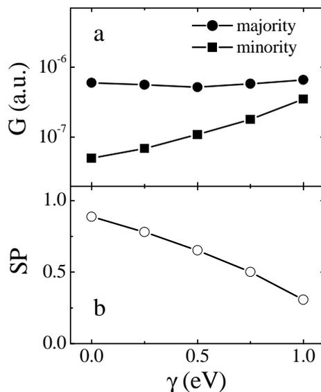
**Fig.16** The calculated conductance for the majority- and minority-spin electrons (a) and the spin polarization (b) of the conductance in a Fe/I/Fe tunnel junction as a function of disorder parameter  $\gamma$ . With increasing disorder the SP decreases due to the contribution from the interface state in Fe. A typical value of  $\gamma$  for sputtered 3d-metal films is about 0.5eV. After Tsymbal [147].
