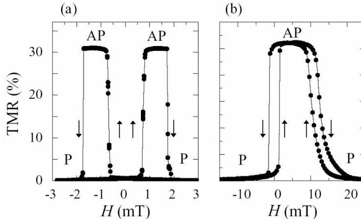
**Fig.6** Magnetoresistance versus magnetic field for a hard-soft MTJ (a) and an exchange-biased MTJ (b), both at 10 K. Vertical arrows refer to sweep direction. Both curves are taken at  $V = 0$ . From LeClair [28].
