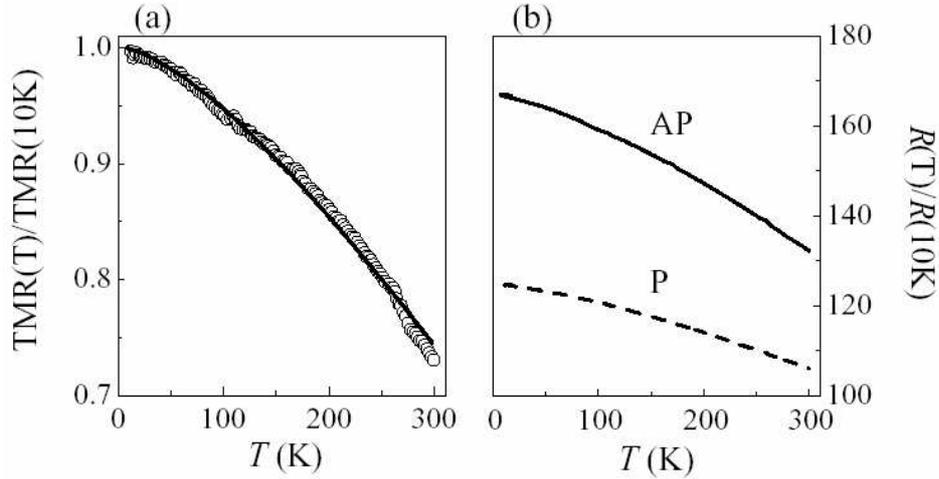
**Fig.8** (a) Temperature dependence of TMR for a Co/Al<sub>2</sub>O<sub>3</sub>/Co MTJ (circles) along with a fit to the model of Shang *et al.* [42] (line). (b) Resistance versus temperature for parallel (P, dashed line) and antiparallel (AP, solid line) magnetization alignment for the same junction. From LeClair [28].
