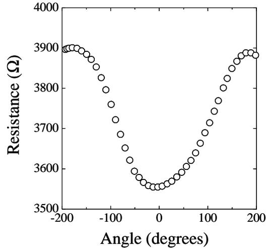
**Fig.7** Angular dependence of the magnetoresistance of a CoFe/Al<sub>2</sub>O<sub>3</sub>/Co junction measured in a magnetic field lower than the coercive field of one electrode but higher than the coercive field of the other electrode. After Moodera and Kinder [29].
