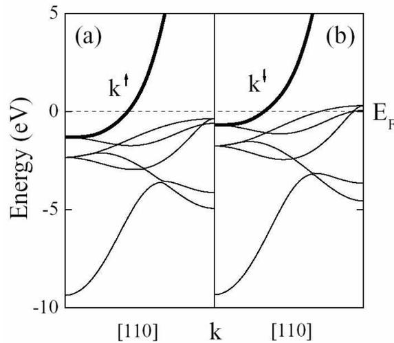
**Fig.3** Electronic bands in bulk fcc Ni in [110] direction for the majority- (a) and minority- (b) spin electrons. The heavy lines show the free-electron-like bands which dominate tunneling.  $k^\uparrow$  and  $k^\downarrow$  are the Fermi wave vectors which determine the spin polarization of the tunneling current. After Stearns [7].
