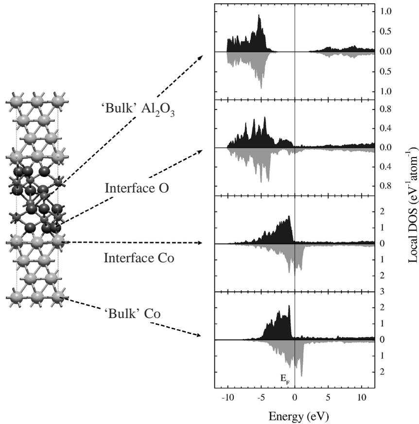
**Fig.14** The calculated atomic structure and local density of states (DOS) for majority-spin electrons (top panels) and minority-spin electrons (bottom panels) for a Co/Al<sub>2</sub>O<sub>3</sub>/Co tunnel junction. After Oleinik *et al.* [127].
