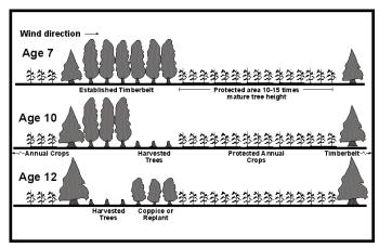
reduction. For maximum wind protection, timberbelts should be spaced across the field at 10 to 15 times the height of the timberbelt at the age it is to be harvested. Specific spacings between timberbelts should be at even multiples of the width of the largest agricultural implements (e.g., sprayers).
