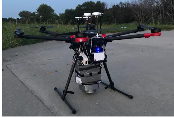
Figure 11. The set-up of UAV (DJI M600 Pro) with the thermal camera (FLIR A8300)
