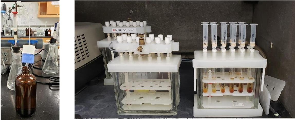
**Figure 12: Left figure SPE Line and Right figure features elution and blowdown of sample**
