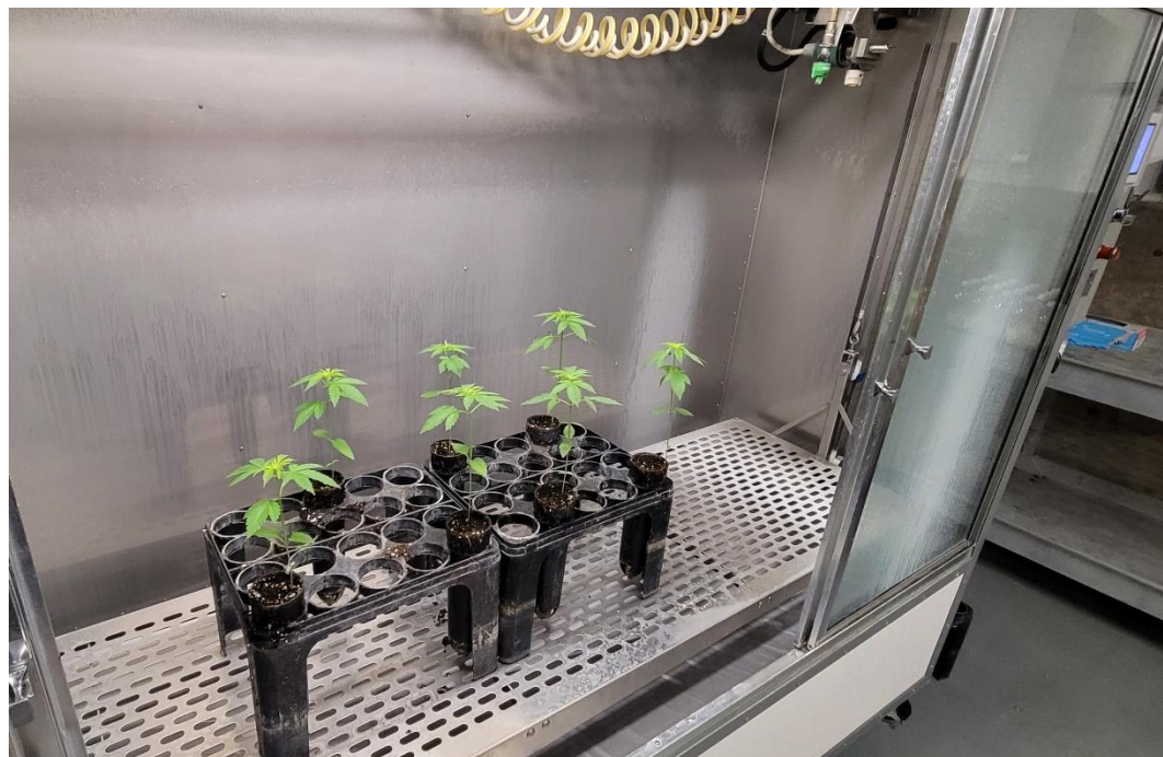
Figure 3.1. Interior of a single-nozzle spray chamber with industrial hemp plants prior to exposure to one of the acetyl-CoA carboxylase inhibitor herbicides tested in the dose response experiment.
