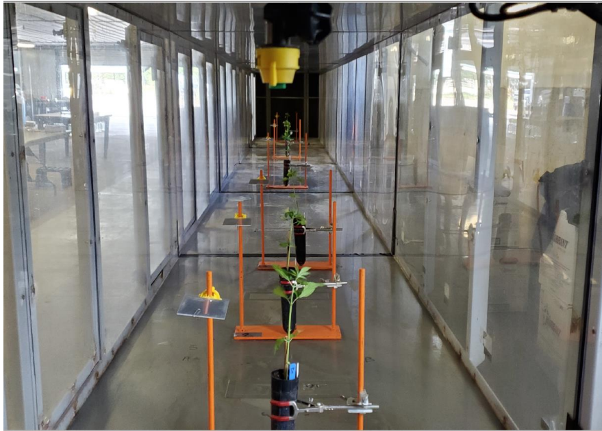
Figure 2.1. Interior of low-speed wind tunnel with spray deposition collectors and industrial hemp plants positioned at downwind distances from the nozzle.
