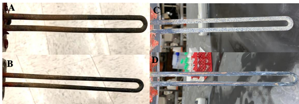
Figure 4.5 Scale formed on heater element from the experiment with a tank with 70.4 in 2 of exposed iron of (A) Untreated water (B) Magnetically treated water, and from the experiment with a tank with little exposure of iron of (C) Untreated water (D) Magnetically treated water
