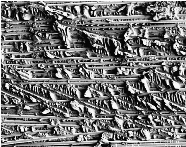
Figure 15. SEM fractographic analysis of 12°/-12° interfaces.
