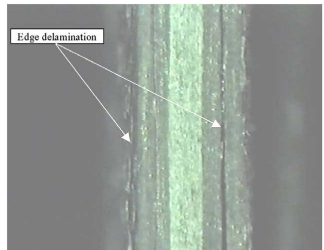
Figure 11. Edge delamination along 12^\circ/-12^\circ interfaces.
