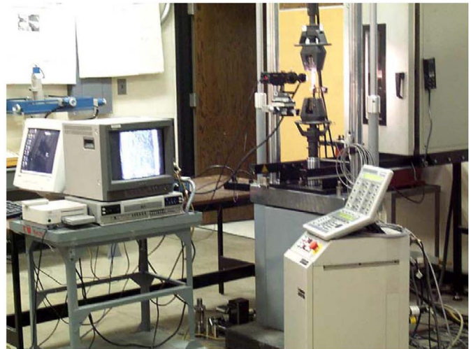
Figure 8. Edge-delamination tensile testing setup.
