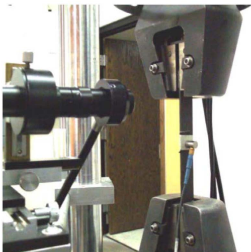
Figure 9. Digital microscopy camera, specimen, AE sensor, and grips.
