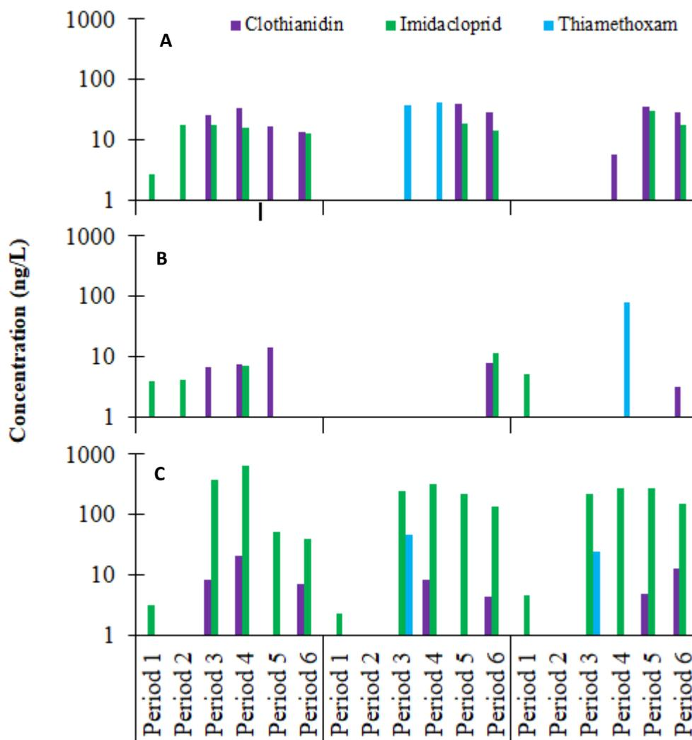
Figure 2.8: Grab pesticide concentrations of clothianidin, imidacloprid, and thiamethoxam at each sampling location in the agricultural (A), herbaceous (B), and urban (C).
