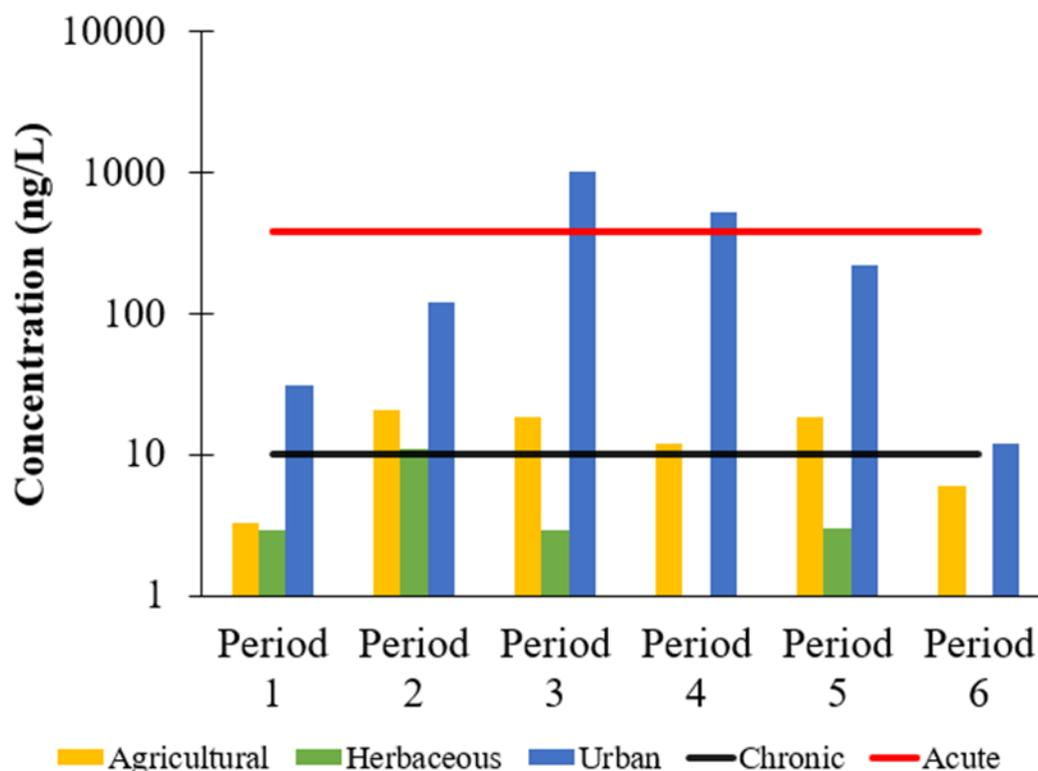
Figure 2.7: Imidacloprid POCIS concentrations at each lake throughout the length of the experiment. \* POCIS membranes for the Herbaceous lake were not viable due to storage complications during Period 4. The red and black lines represent chronic and acute toxicity respectively.
